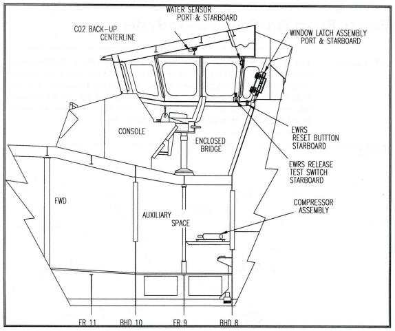
Figure 3-14 Emergency Window Release System
