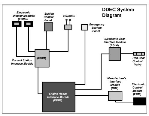
Figure 3-3 DDEC System Diagram
