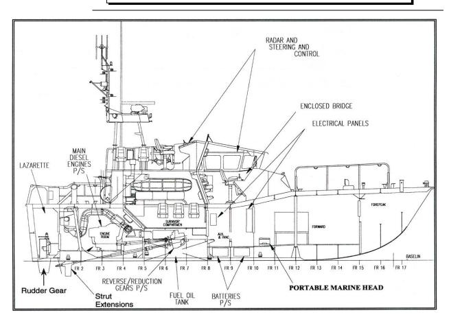
Figure 2-2 47FT MLB Inboard Profile
