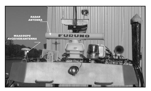
Figure 3-24 Radar Antenna WAAS/DGPS Receiver/Antenna
