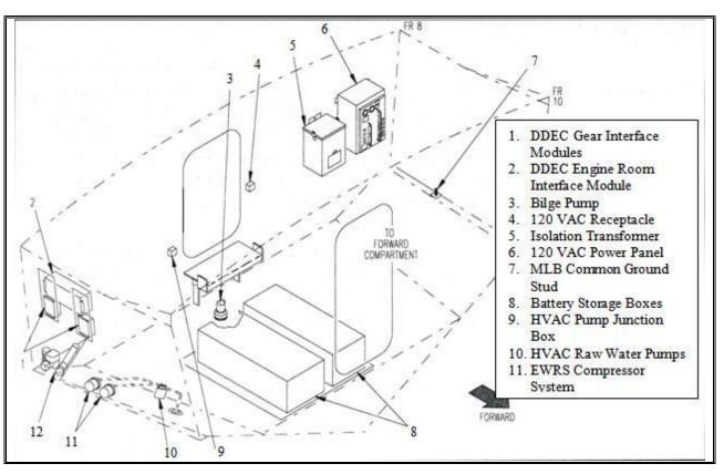
Figure 2-5 Auxiliary Machinery Compartment, Aft View
