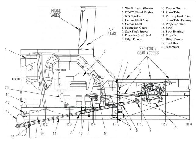
Figure 3-1 Propulsion System (Engine Room & Survivors Compartment)
