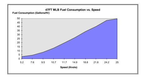
Figure 5-1 Fuel Consumption vs. Speed
