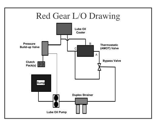
Figure 3-2 Reduction Gear Lube Oil Drawing
