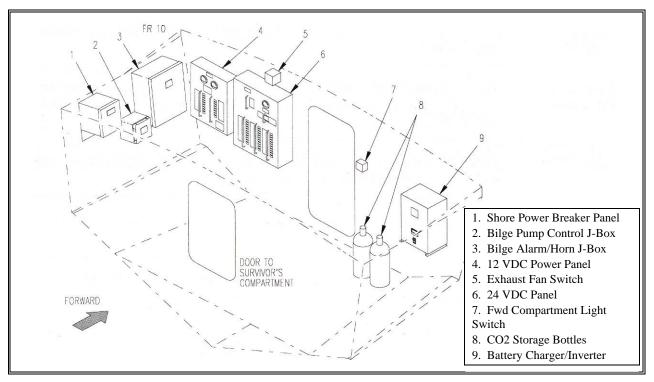
Figure 2-4 Auxiliary Machinery Compartment, Forward View
