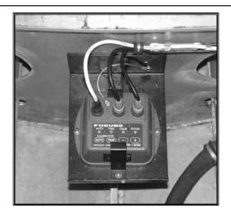
Figure 3-27 Heading Sensor
