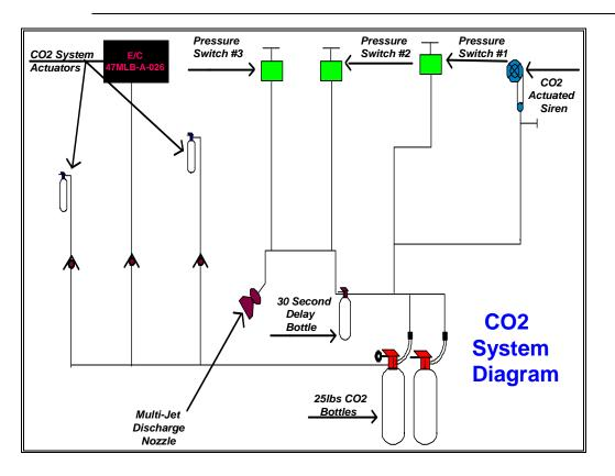
Figure 3-15 Engine Room Fire Suppression System
