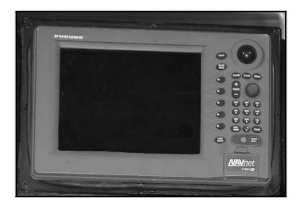
Figure 3-23 Radar Display
