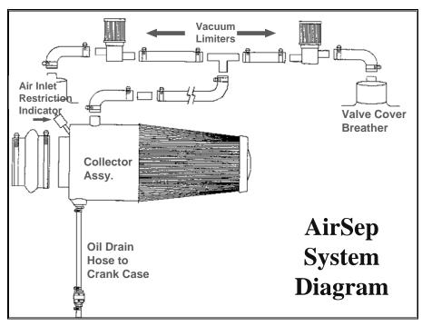
Figure 3-6 AirSep System Diagram
