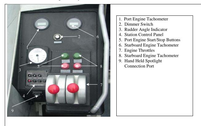
Figure 2-14 Open Bridge, Port Steering Station
