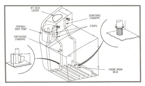
Figure 3-17 Dewatering & Fire Fighting Standpipes
