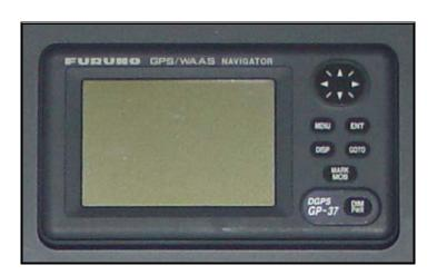
Figure 3-26 GP-37 WAAS/DGPS Receiver and Navigator
