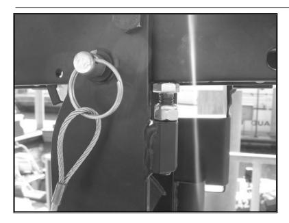
Figure 3-30 MK-97 Locking Nut
