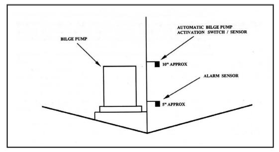
Figure 3-18 Bilge Flood Alarm System
