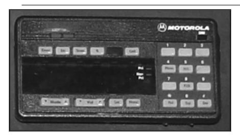
Figure 3-20 Motorola VHF-FM Astro Spectra W9 Transceiver Control Head
