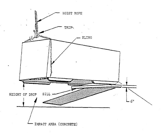
Figure 1. Edgewise drop (Rotational)
