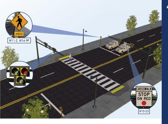
A Pedestrian Hybrid Beacon head consists of two red lenses above a single yellow lens. Unlike a traffic signal, the PHB rests in dark until a pedestrian activates it via pushbutton or other form of detection. When activated, the beacon displays a sequence of flashing and solid lights that indicate the pedestrian walk interval and when it is safe for drivers to proceed (see figure on back page).
