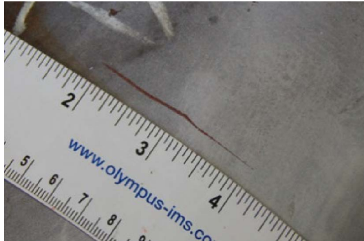
Figure 2. Transportation Technology Center, Inc. (TTCI) cracked axle (Axle 1822)
