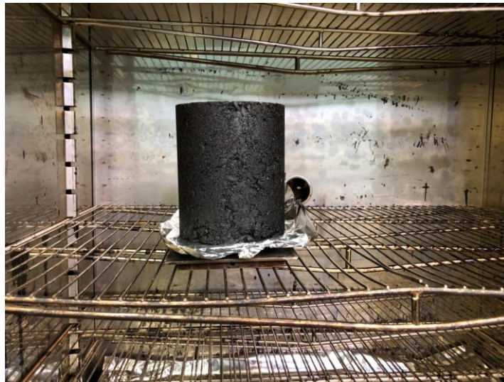
Figure F.1. Compacted 180mm pills aging in a forced-draft oven.
