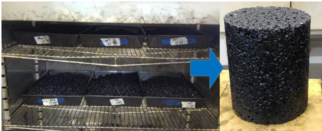
Figure 3.8. Loose mixture aging.
