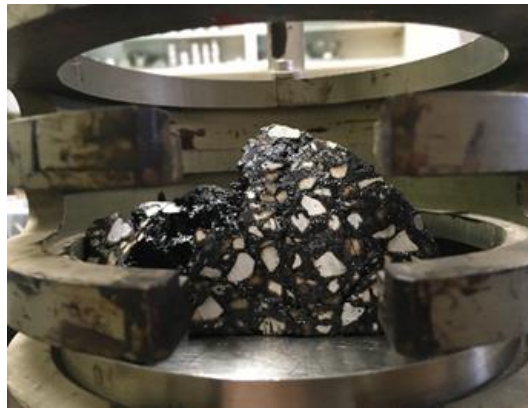
Figure 4.1. I-FIT specimen deformed after PAV aging.
