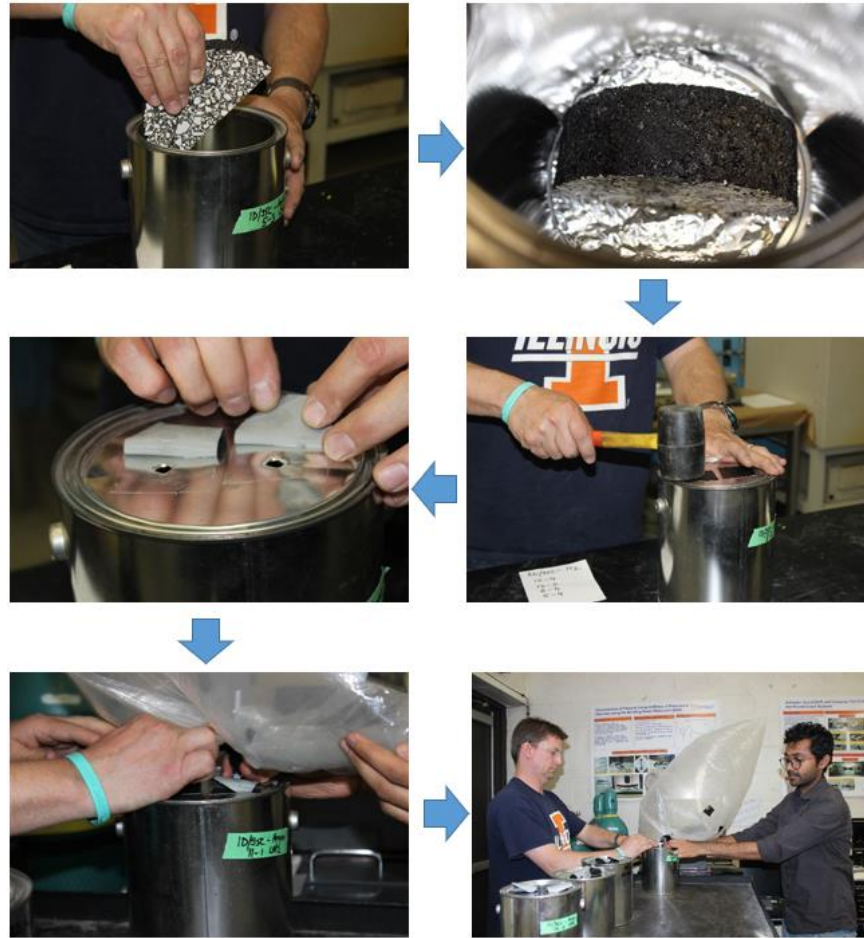
Figure 4.16. Preparation process for argon aging.
