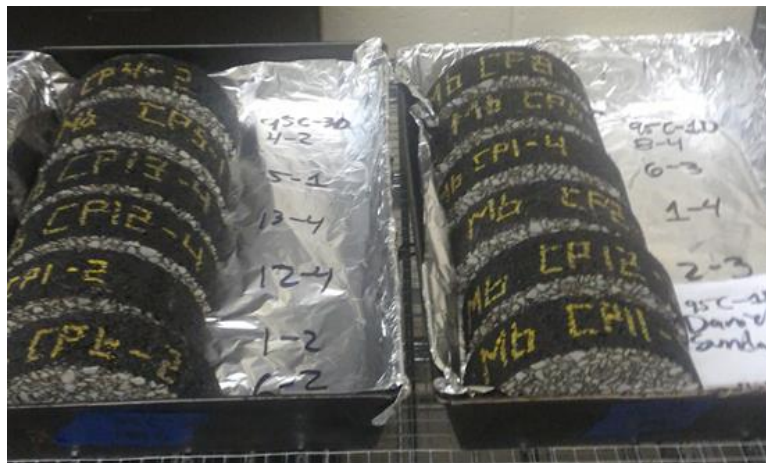
Figure 3.17. Trays containing specimens ready for aging process.
