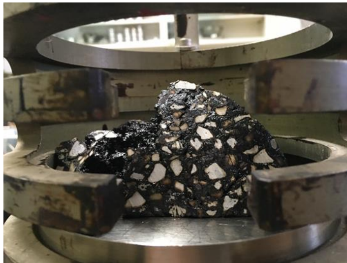
Figure 3.10. I-FIT specimen after PAV aging.
