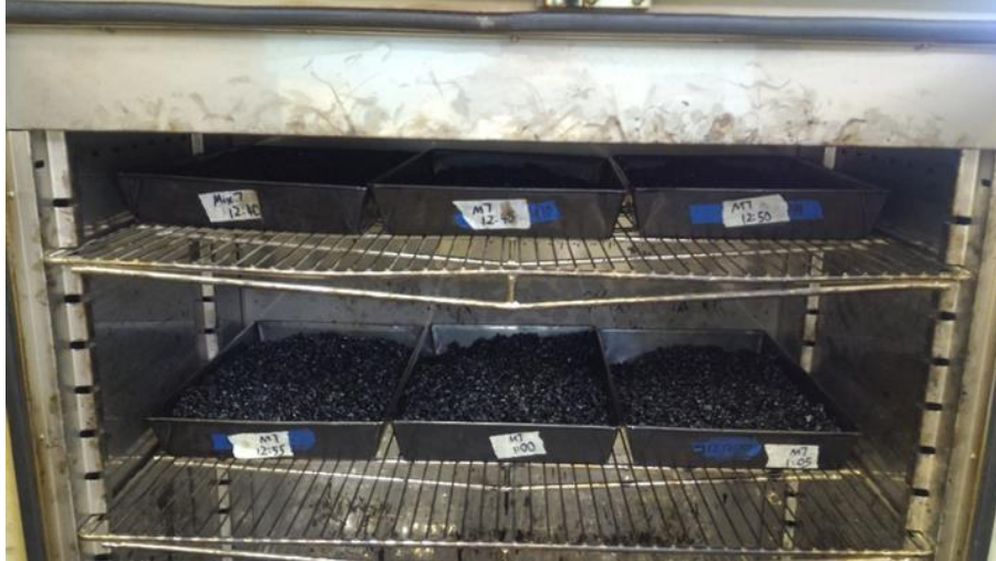
Figure 3.14. Conditioning of batched samples before compaction.
