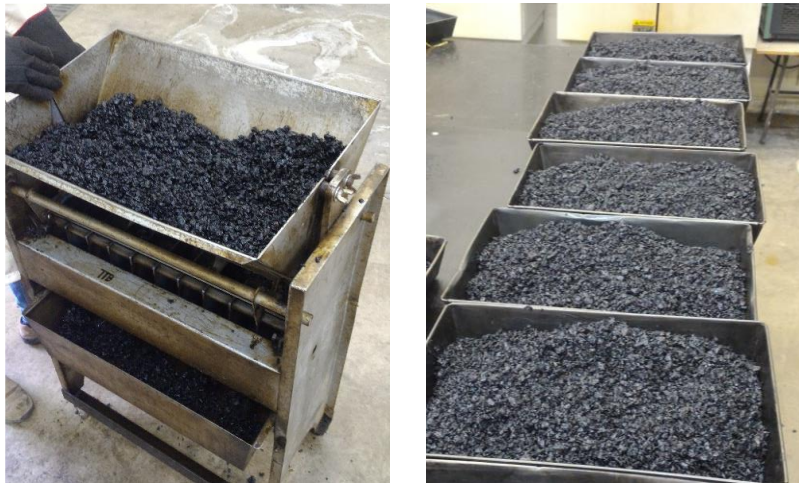
Figure 3.13. Material splitting and batched samples.
