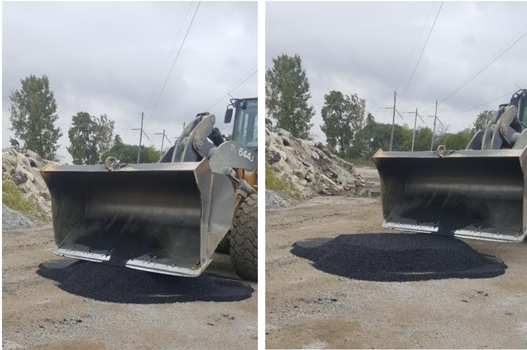
Figure 3.3. Spread the sample to flatten conical heap.
