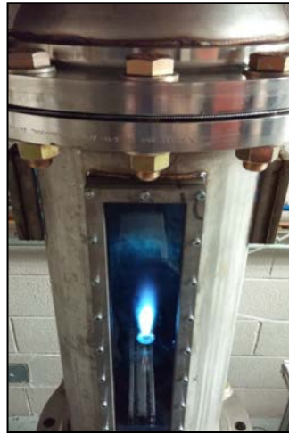
Figure 13. Photograph of a flame in a pressure vessel under subatmospheric conditions.
