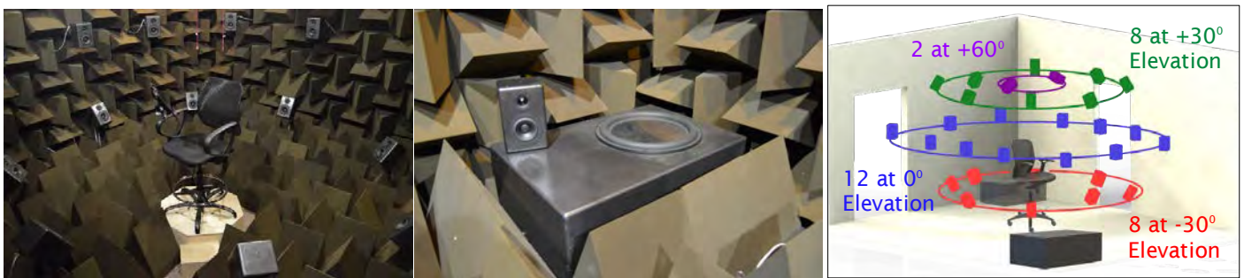
Figure 21. The AURAS facility at Penn State. The photo on the left shows the anechoic chamber as set up for testing. The center image shows the subwoofers with a two-way loudspeaker included for scale. The final image on the right shows a schematic of the arrangement of the loudspeaker positions around the central listening point.
