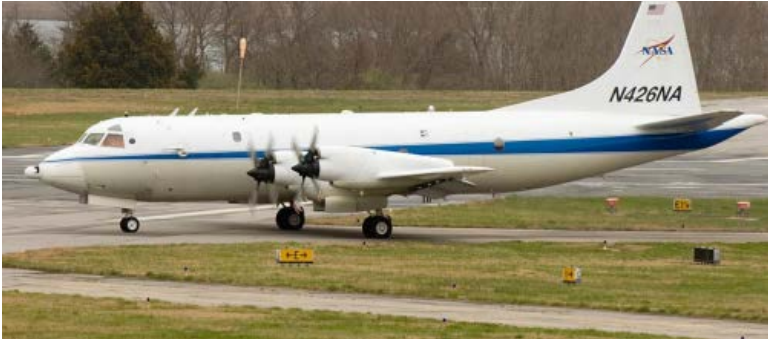
Figure 12. Lockheed P-3B Orion four-engine turboprop aircraft used in the experiment.
