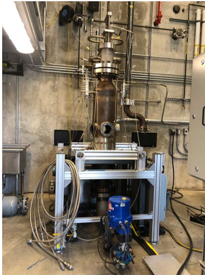
Figure 3. Photograph of the variable ambient pressure spray (VAPS) test rig.
