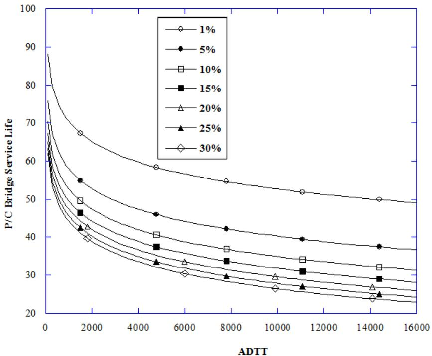
**Figure 16: Estimated service life of PC multibeam bridge per % of overweight truck.**
