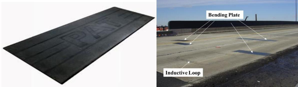
**Figure 4: Bending plate and installation example (<https://www.irdinc.com>; Nassif et al., 2005).**
