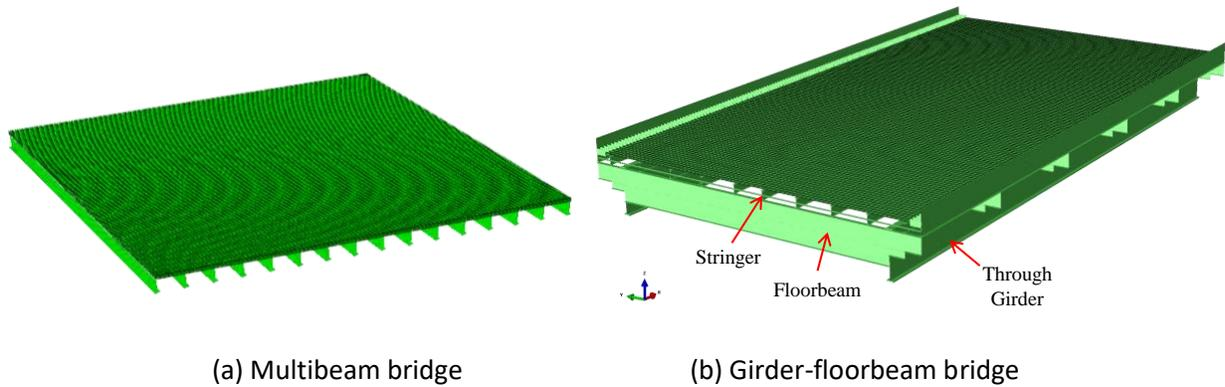
**Figure 14: Finite Element (FE) models for steel bridges.**
