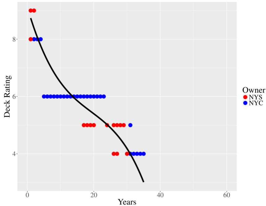
**Figure 18: Deck condition rating time series for all bridges near AHB.**
