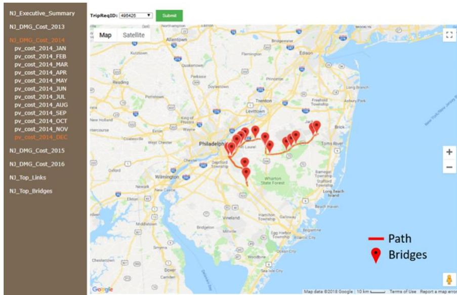
**Figure 12: Graphical User Interface of Developed GIS Application for NJ Permit**
