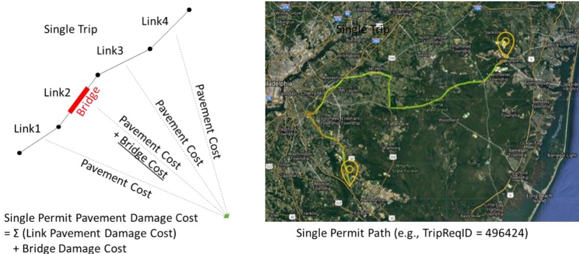
**Figure 9: Pavement damage cost calculation procedure of single overweight permit trip.**
