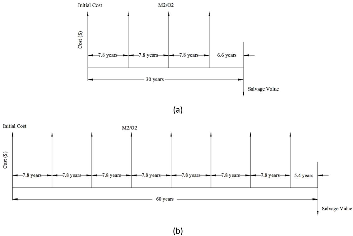
**Figure 11: Activity flow with pavement service life of 7.8 years in (a) 30-year and (b) 60-year analysis period (Nassif et al., 2015).**
