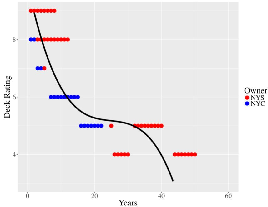
**Figure 22: Deck condition rating time series for all bridges near RKW.**
