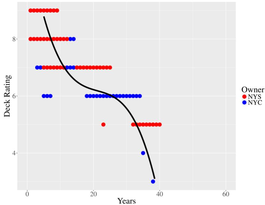
**Figure 20: Deck condition rating time series for all bridges near VDM.**
