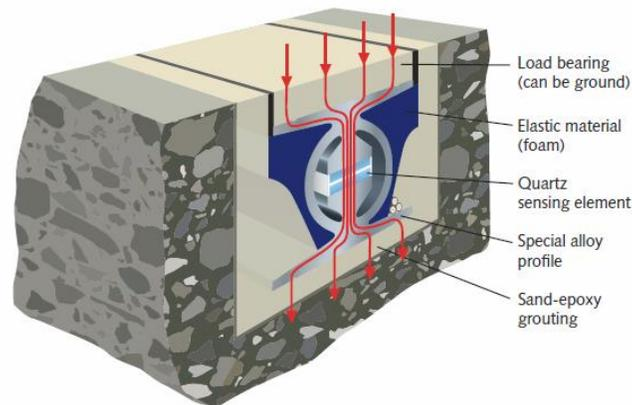
**Figure 2: Quartz sensor (<https://www.traffic-data-systems.net>).**
