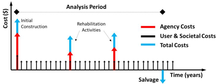
**Figure 10: Conceptual cash flow diagram of a project (Kaan et al., 2004).**
