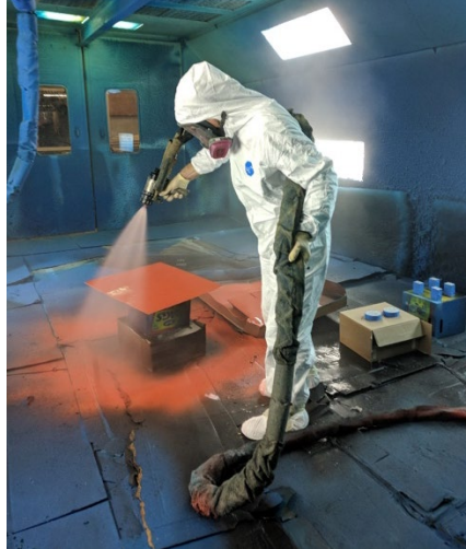
Figure 4.1 Polyurea spraying at a local supplier (VersaFlex®).
