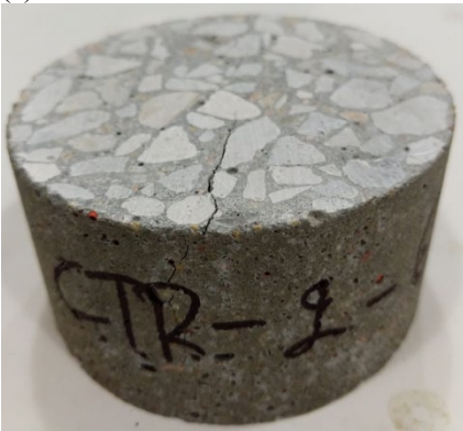
Figure 4.5 Impact test results: (a) acceleration vs. time at impact, (b) cracks in uncoated specimen (control) and (c) coated specimens after two impact testings.
