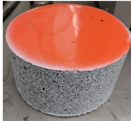
Figure 4.5 Impact test results: (a) acceleration vs. time at impact, (b) cracks in uncoated specimen (control) and (c) coated specimens after two impact testings.
