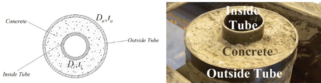
Figure 2.21 Concrete-filled double skinned tube (84)
