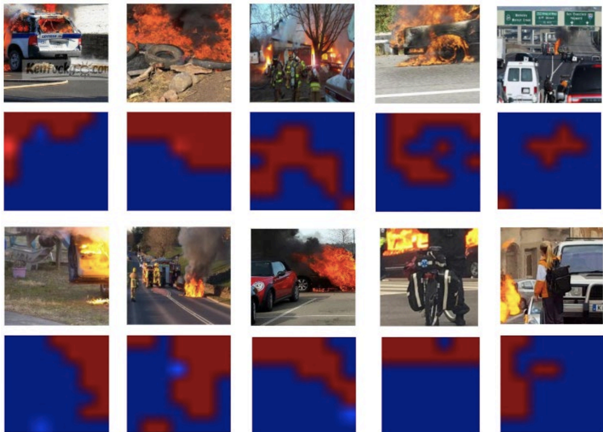
Figure 4.1 Visualization of our spatial attention map. Our spatial attention model learns to locate the fire and accident regions in the image.
