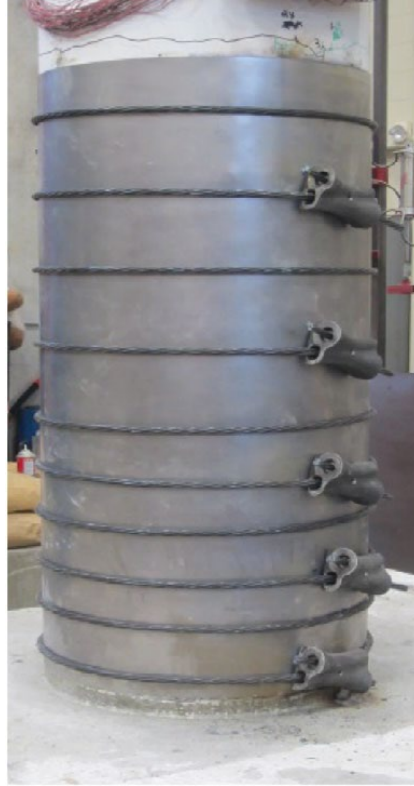
Figure 5.2 Column repaired with hybrid steel jacket (Fakhairifar et al 2015a)
