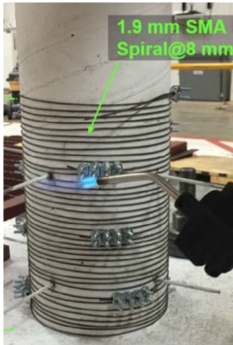
Figure 5.4 SMA active confinement (Jung et al. 2018)
