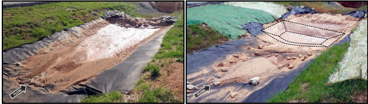
(a) inflow channel without excavated sump (S1)
