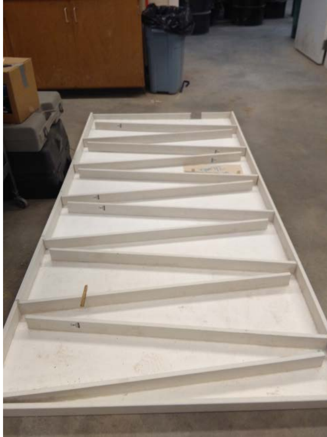
Figure 4.13: Mixing tank unit constructed for the addition and mixing of flocculant in inflows reaching the small-scale lamella settler (SSLS) unit.
