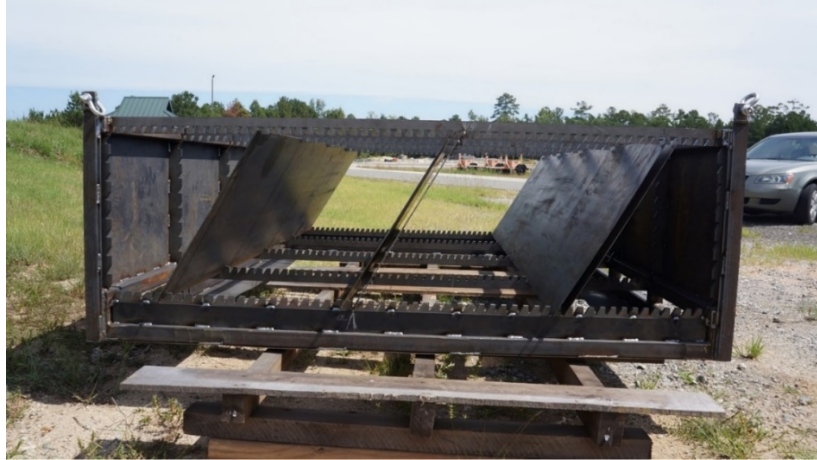
(a) Lower portion of a high-rate lamella settler unit
