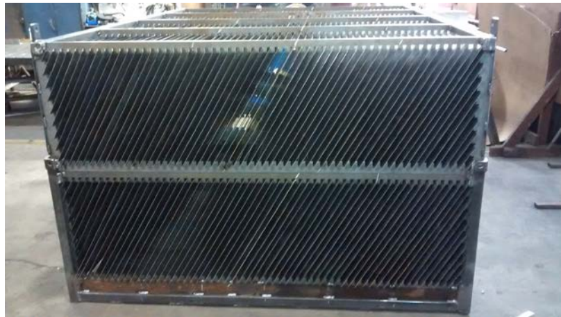
(b) Lower and upper portion of a high-rate lamella settler unit, with lamella plates installed
