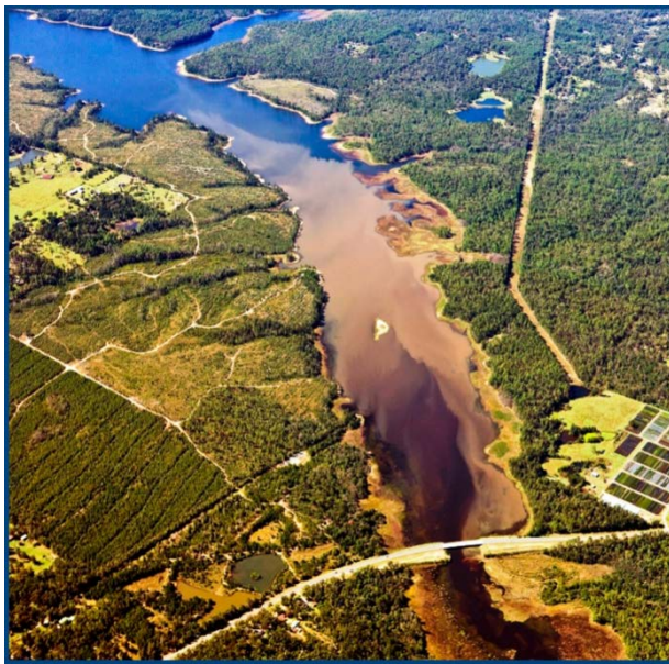
Figure 1.1: Example of a sediment plume resulting from road construction runoff (Clark et al., 2012)
