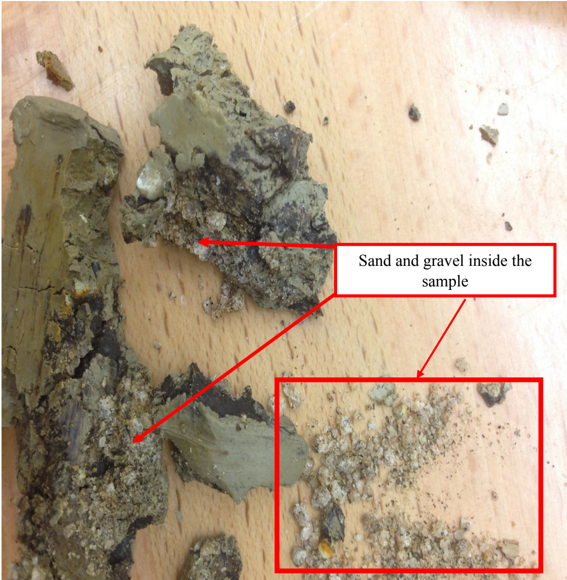
Figure 5.6 Sand particles inside of sample IS-19.5 (I-180 and Superior St.)
