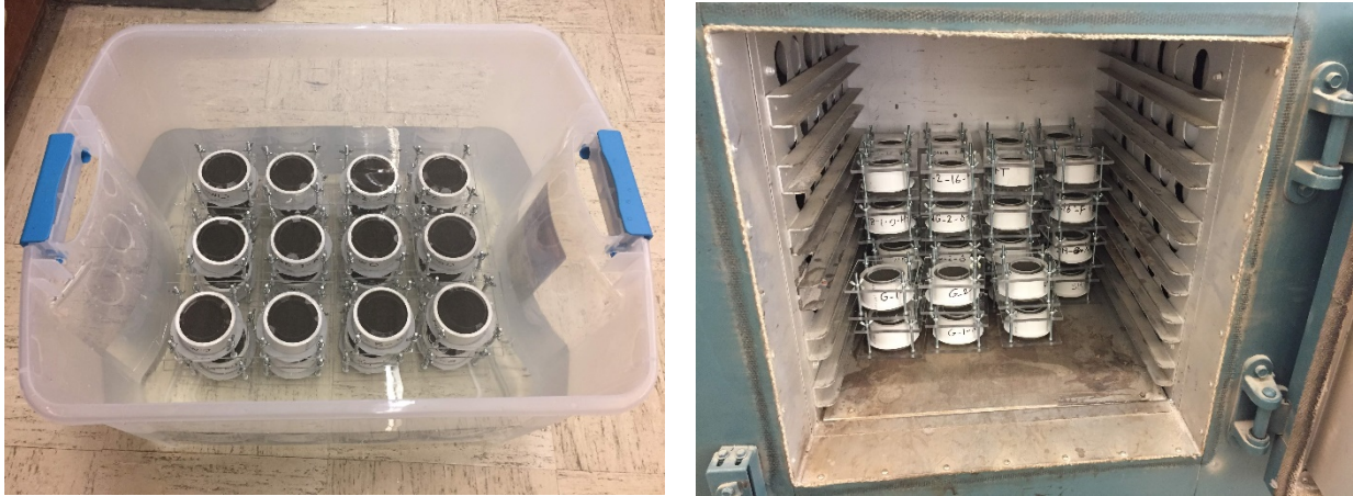
Figure D.10 Water bath and oven used for weathering soil samples
