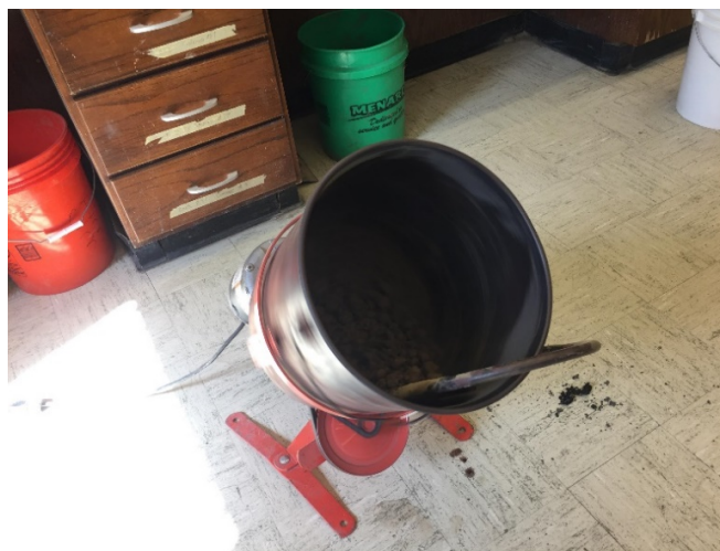
Figure D.1 mixing soil with biopolymers and water
