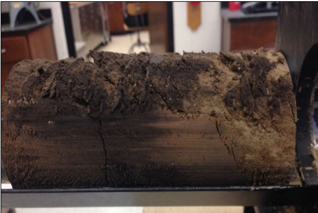
Figure 4.5 Cracks on sample NL-14.5
