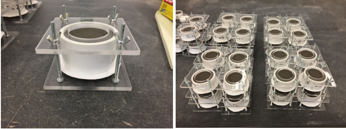
Figure D.9 Securing samples in the fixture for weathering
