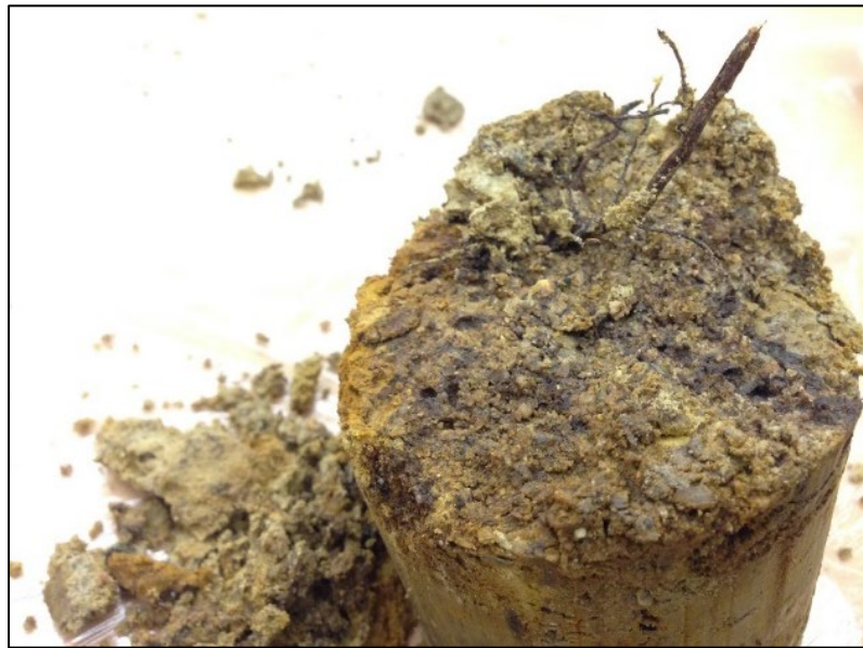
Figure 4.4 Non-uniformity and cracks in Sample IS-14.5 (I-180 and Superior St.)
