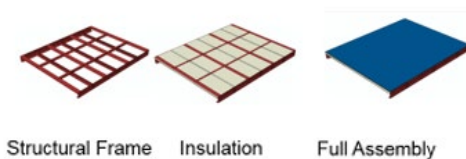
Figure 1. ABAQUS model showing component geometry of Design 1
