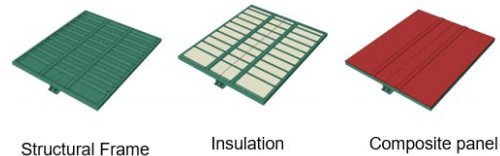
Figure 2. ABAQUS model showing component geometry of Design 2
