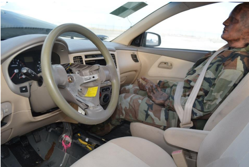
Figure 209. Occupant Compartment Damage, Test No. APR-2
