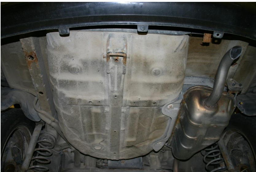
Figure 210. Vehicle Undercarriage Damage, Test No. APR-2
