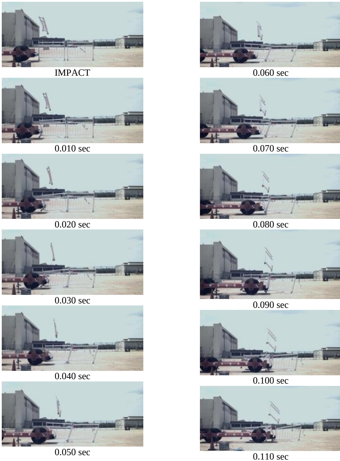
Figure 137. Time-Sequential Photographs, Run No. WIPR-2, Test No. WIPR-2-2
