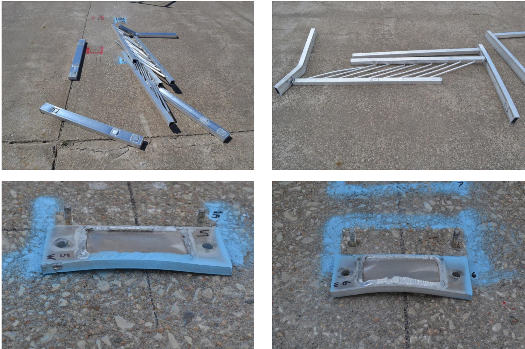
Figure 132. First Panel Damage, Run No. WIPR-1, Test No. WIPR-1-2
