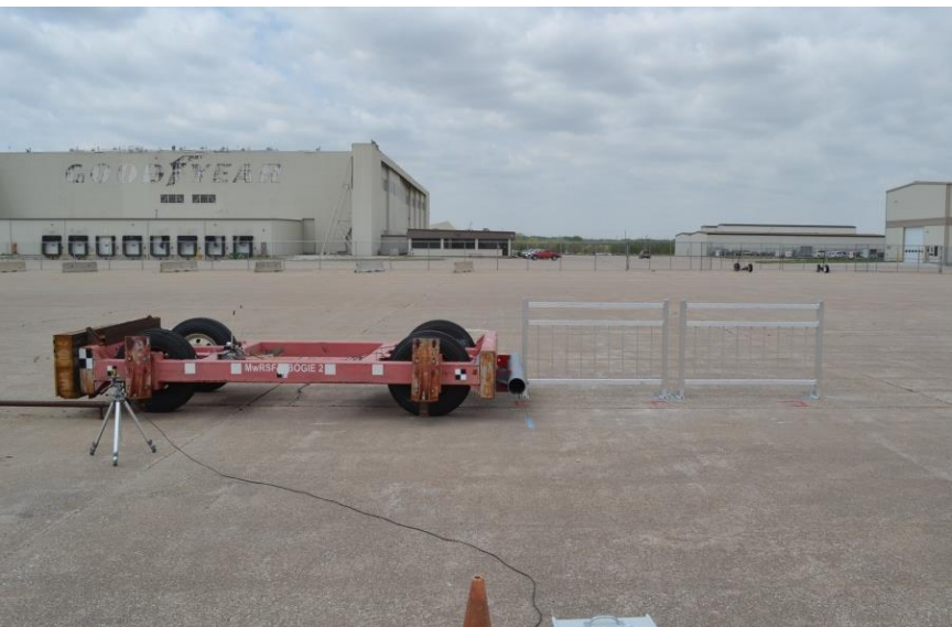
Figure 126. Typical Bogie Testing Setup
