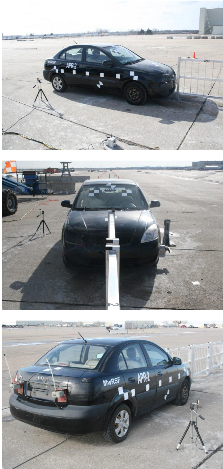
Figure 194. Impact Location, Test No. APR-2
