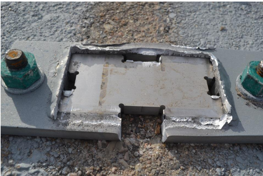
Figure 186. Panel No. 15 Damage, Test No. APR-1
