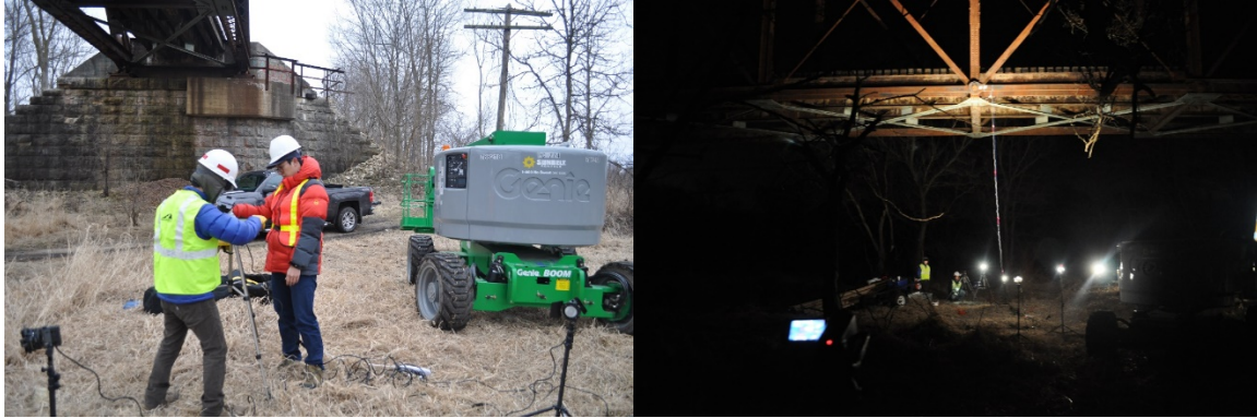
(a) (b) Figure 6.15 (a) Camera and (b) lights setup
