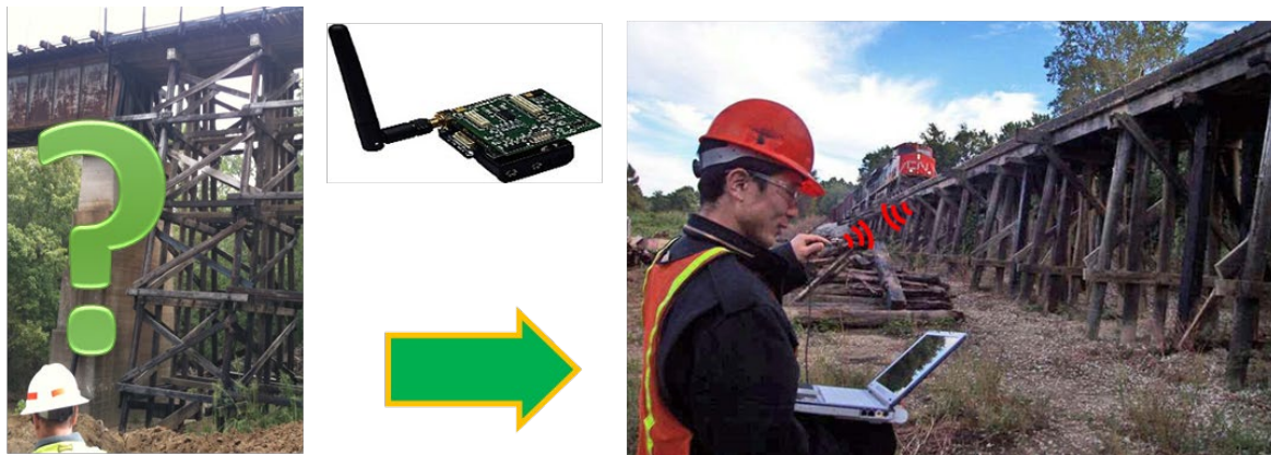
Figure 1.4 Concept of real-time reference-free displacement estimation of railroad bridges under revenue service traffic using WSS
