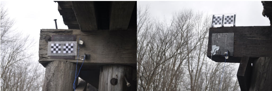
Figure 6.3 Sensors and target at (a) pier 7 and (b) pier 6
