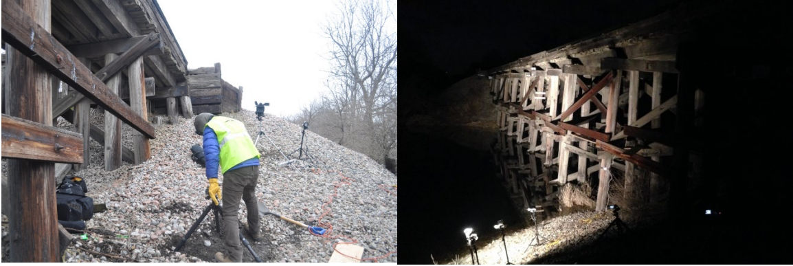
Figure 6.4 Cameras and lights setup
