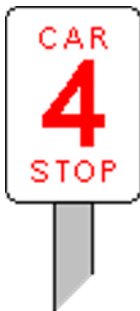
Example of the train stop sign instructing the crew where to stop the train according to car length.
