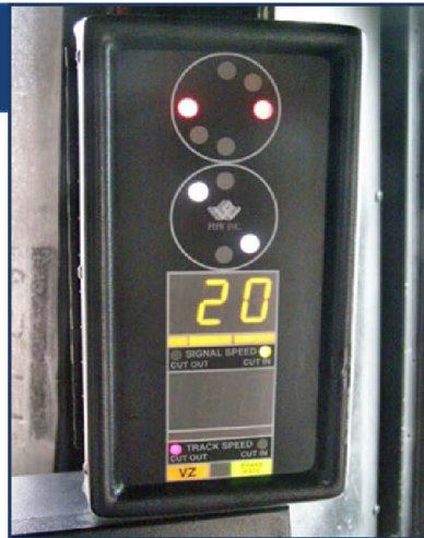
Figure 10. Example cab signal used in passenger operations
