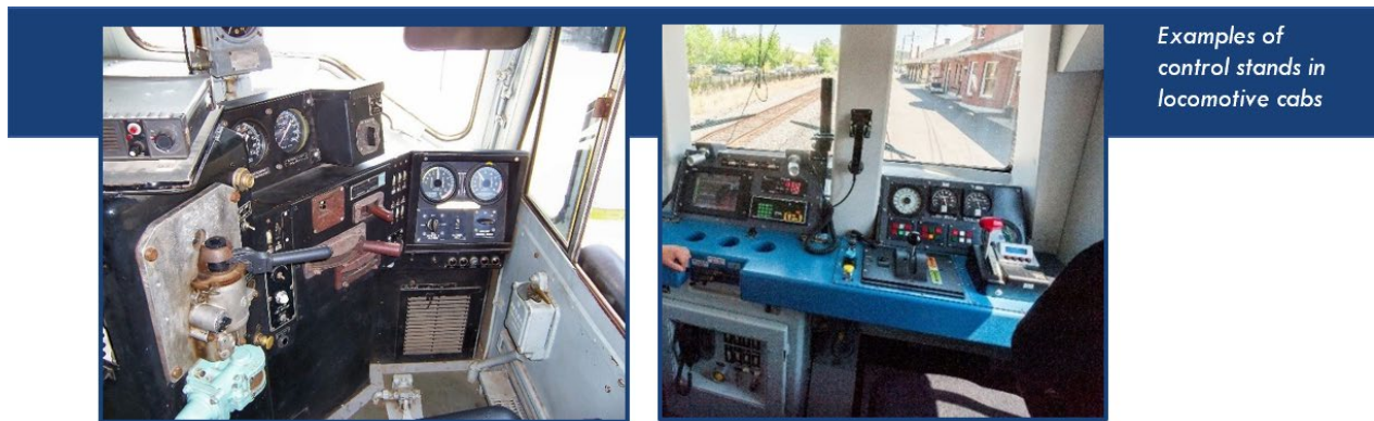
Figure 13. Example of control stands in locomotive cabs
