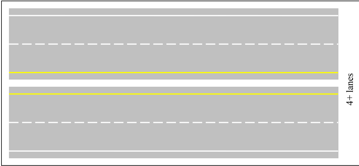
Figure 2. Rural Interstate, Urban Interstate, Urban Other Freeway and Expressway Striping Configuration.
