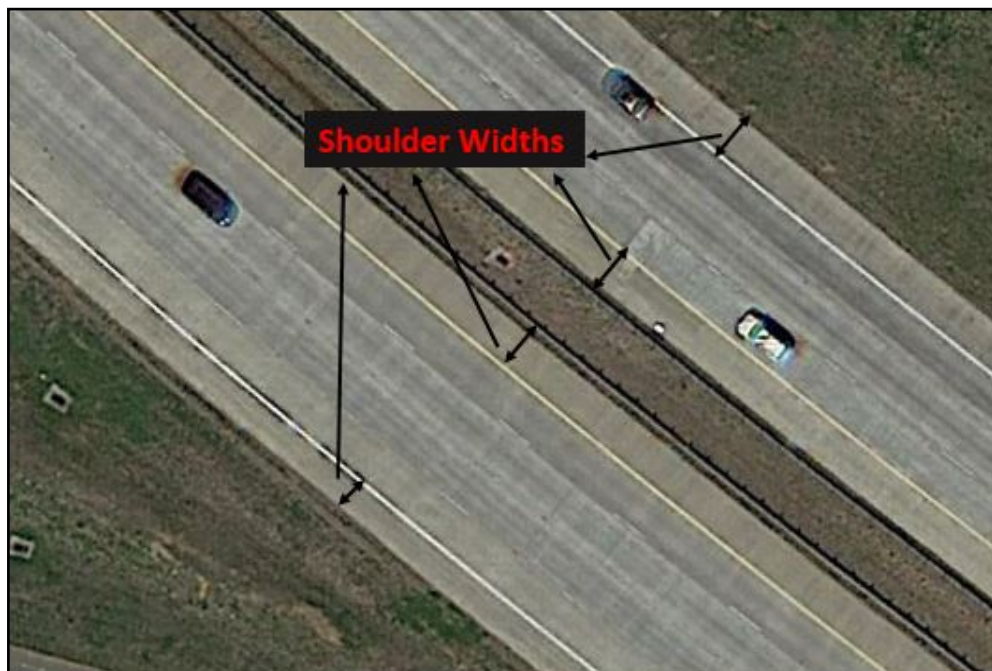
Figure 4. Capturing Shoulder Widths Using Google Earth Pro
