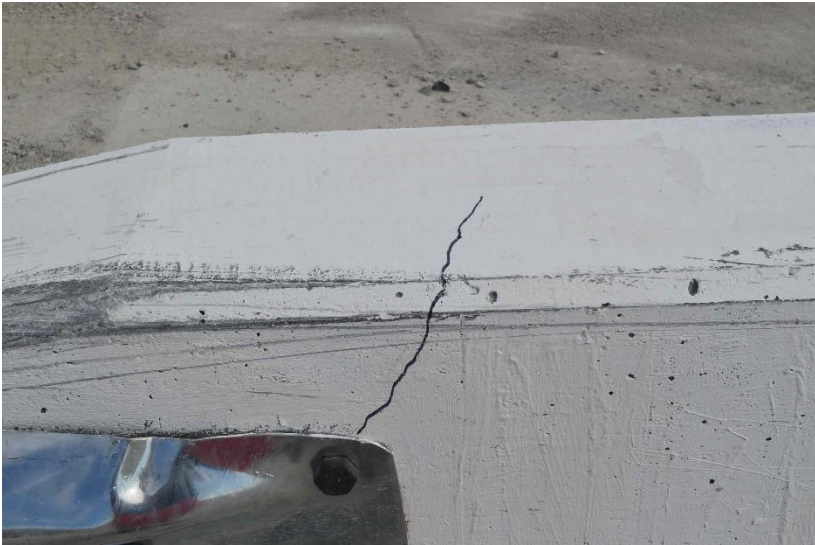
Figure 49. Buttress Damage, Test No. 34AGT-1
