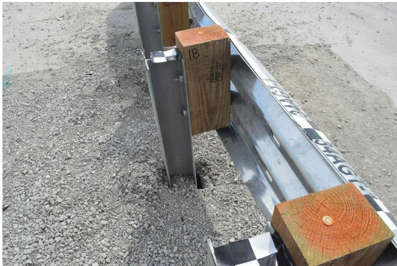
Figure 47. System Damage, Post nos. 16 through 18, Test No. 34AGT-1
