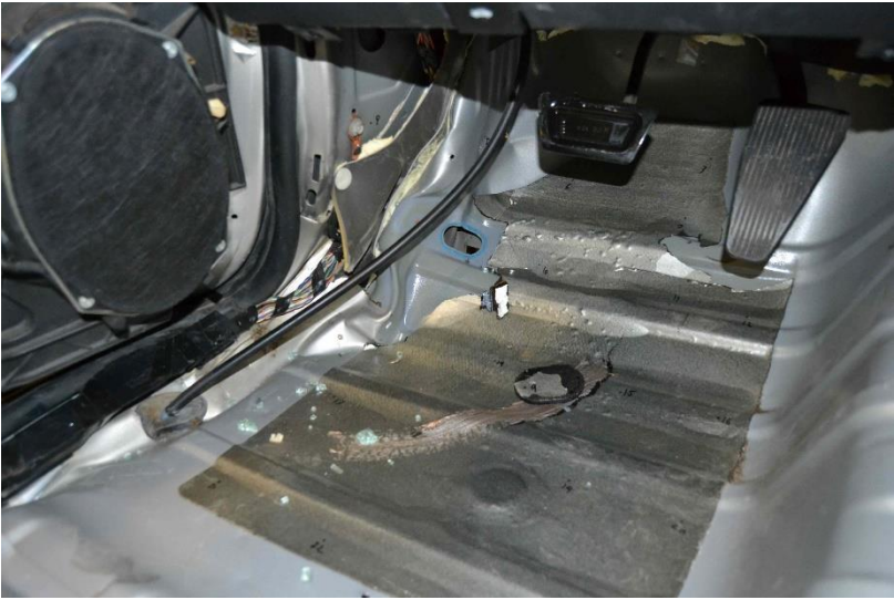
Figure 52. Windshield Damage and Occupant Compartment Deformation, Test No. 34AGT-1
