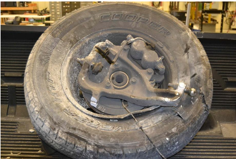
Figure 53. Undercarriage Damage, Test No. 34AGT-1
