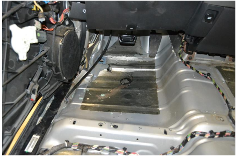
Figure 52. Windshield Damage and Occupant Compartment Deformation, Test No. 34AGT-1
