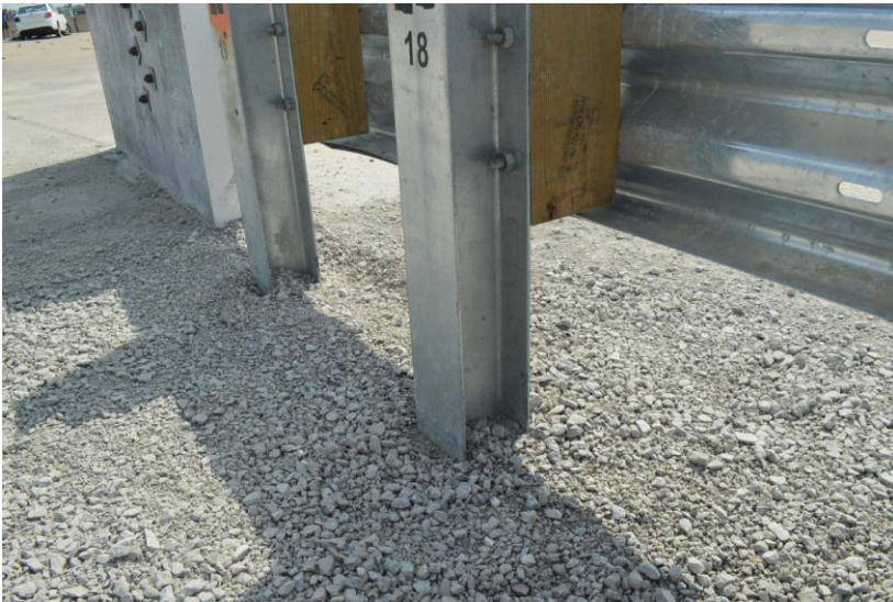
Figure 61. System Damage, Post Nos. 18 and 19, Test No. 34AGT-2
