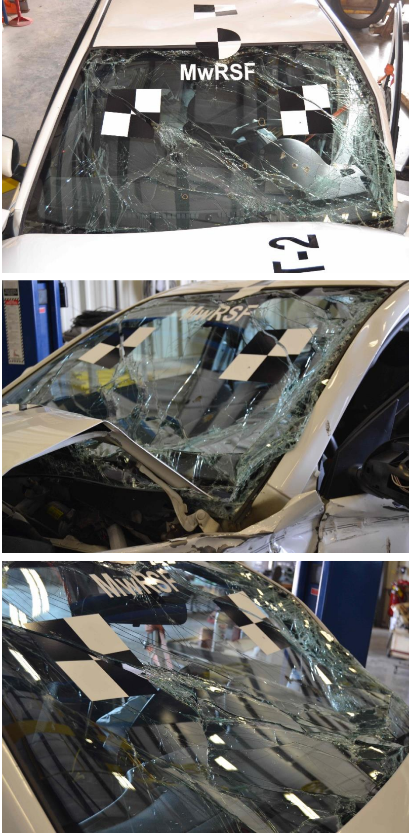
Figure 66. Windshield Damage, Test No. 34AGT-2
