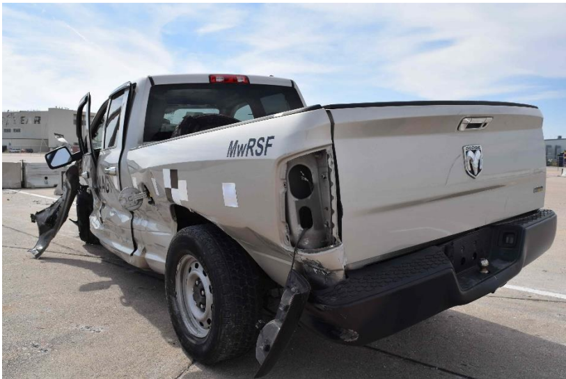
Figure 51. Vehicle Damage, Test No. 34AGT-1
