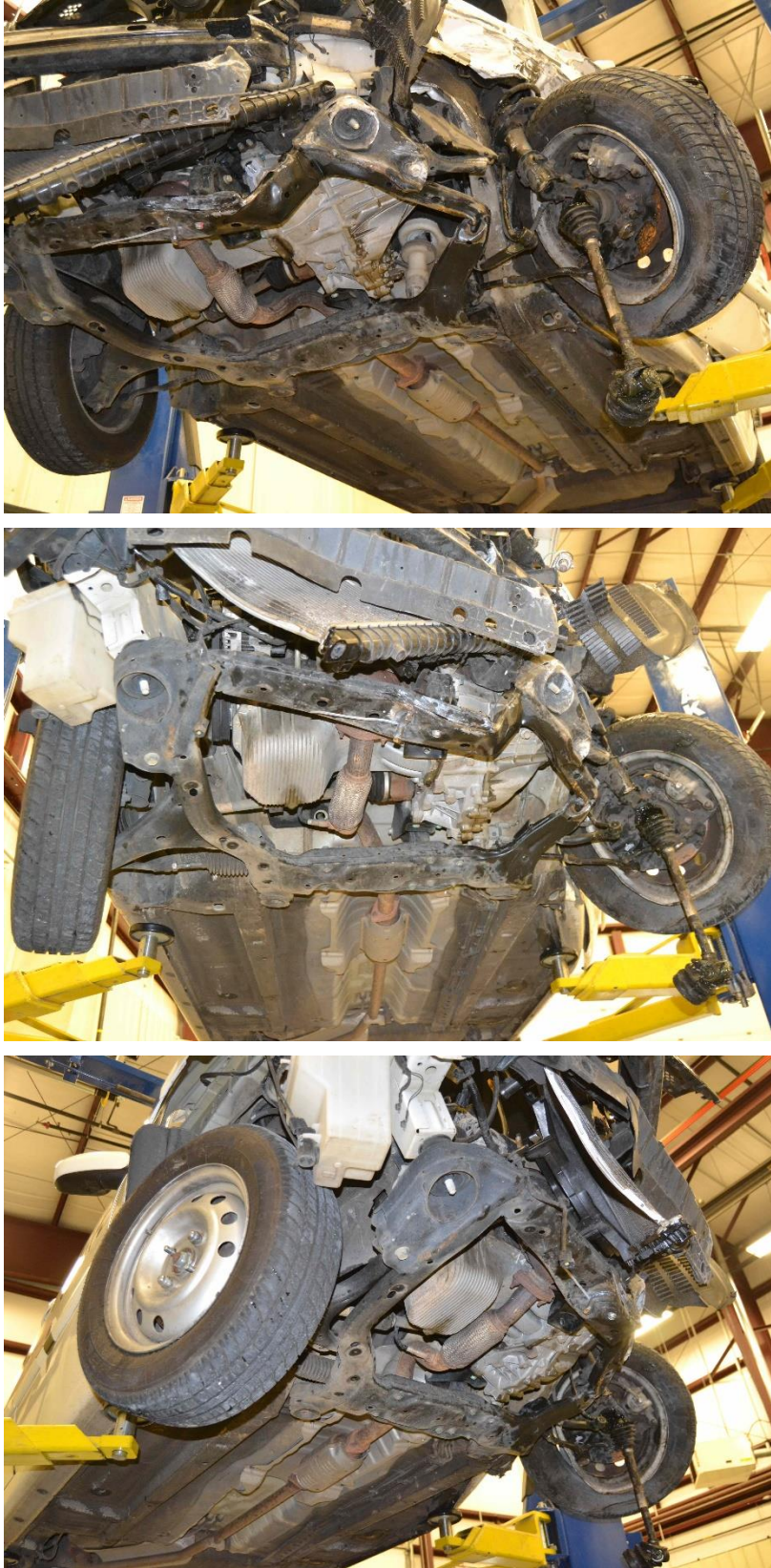
Figure 68. Undercarriage Damage, Test No. 34AGT-2
