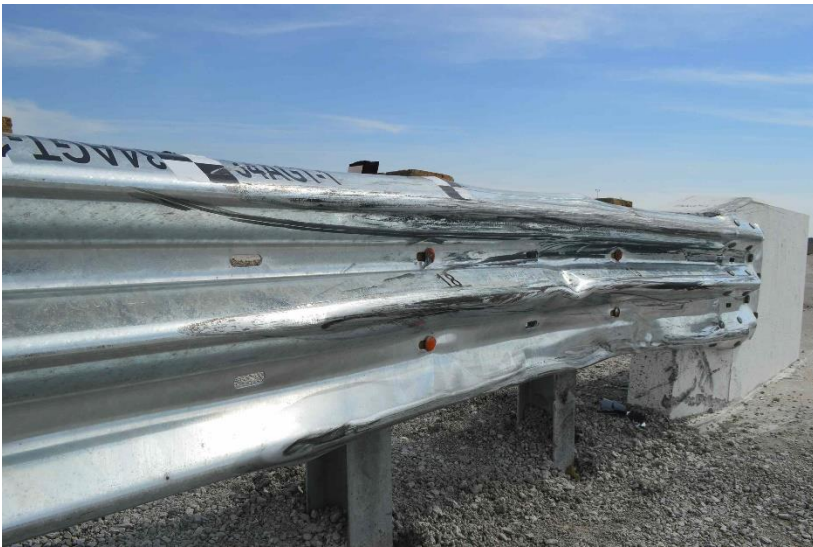
Figure 46. System Damage, Test No. 34AGT-1
