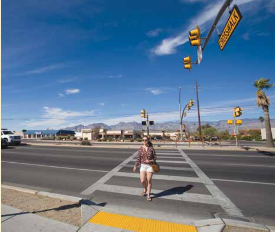
This pedestrian is crossing at a PHB on a wide arterial road. Photo: Martha Lochert Photography.
