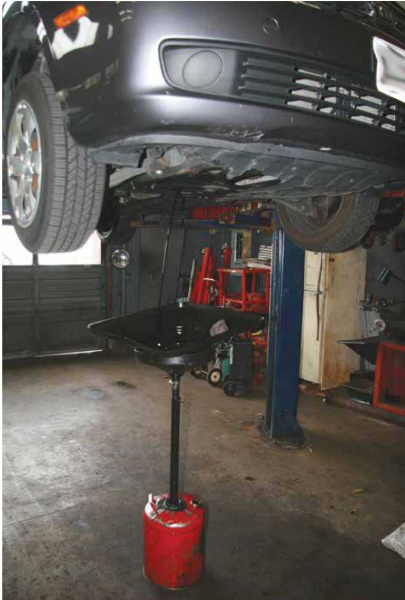
During an oil change, the waste engine oil drains from a car, as shown here.
