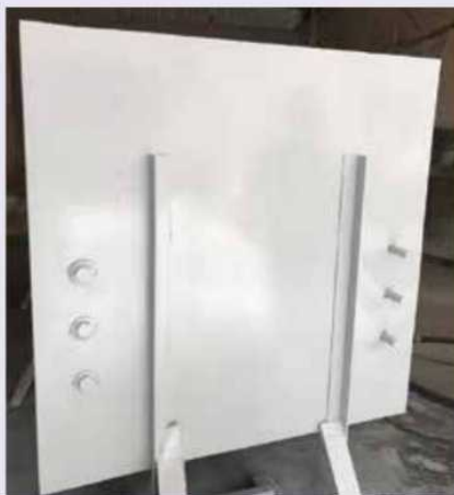
MoDOT tested an innovative protective coating, developed by the oil industry, to assess its performance for use on bridges. Shown here is the steel test plate before (left) and after the application. Photos: Tesla NanoCoatings.
