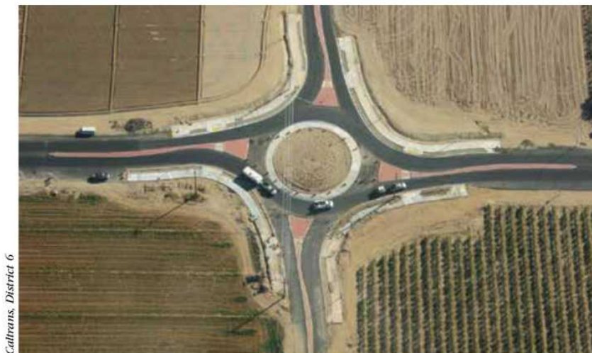
This aerial photograph shows a rural roundabout on State Route 145 in Fresno, CA. The roundabout, connecting SR-145 and Jensen Avenue, features high-speed approaches.
