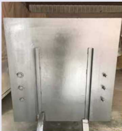
MoDOT tested an innovative protective coating, developed by the oil industry, to assess its performance for use on bridges. Shown here is the steel test plate before (left) and after the application. Photos: Tesla NanoCoatings.
