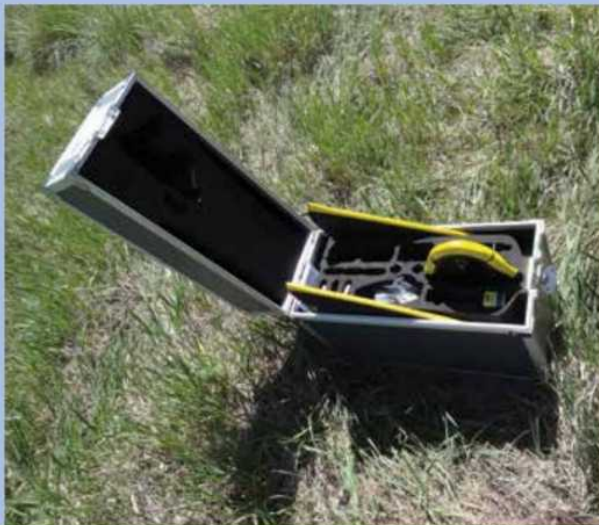
This small unmanned aircraft, disassembled and stored in a box, is one that FHWA's Western Federal Lands Highway Division has tested. It is a basic, fixed mono-wing aircraft and has few moving parts.
