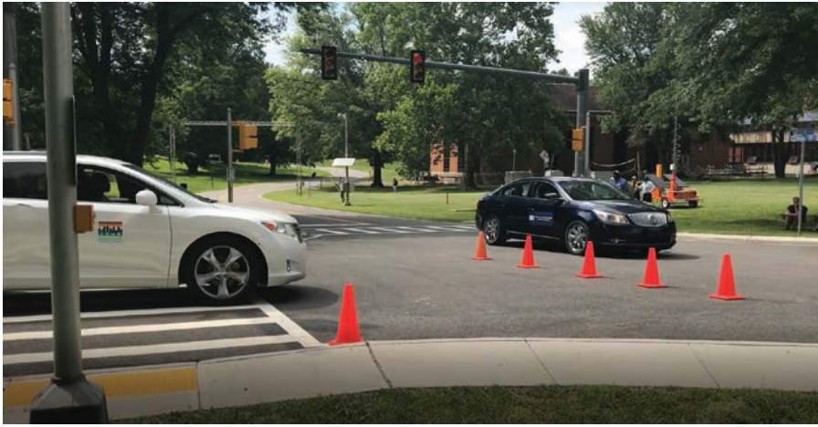
A THEA vehicle (white car) waits as it receives an intersection movement assist warning being triggered by a New York City vehicle (black car) at the TFHRC test track. Photo: USDOT.
