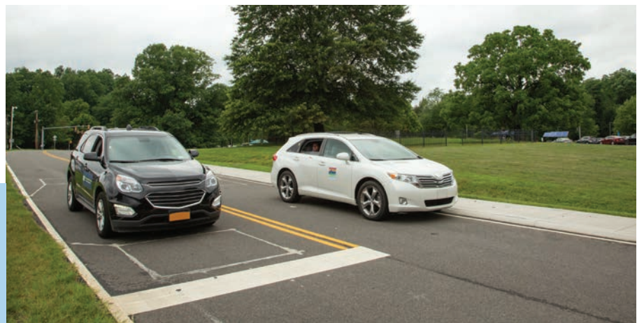
A THEA vehicle (white car) drives in an adjacent lane on a controlled test track at TFHRC without triggering a forward collision warning alert from a stationary NYCDOT vehicle. Photo: USDOT.
