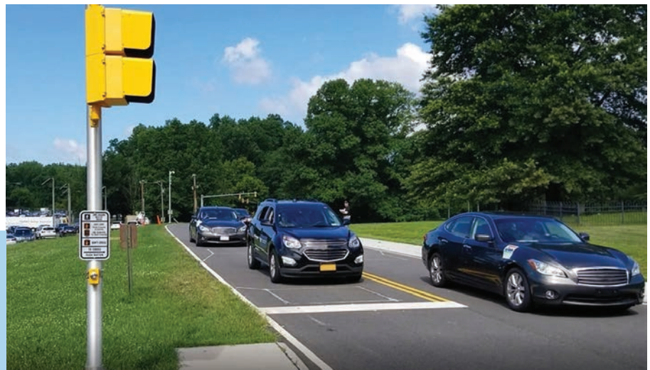
A Wyoming vehicle (on right) receives a forward collision warning alert being triggered by a New York City vehicle with the other four vehicles driving by the adjacent lane on the test track. Photo: USDOT.
