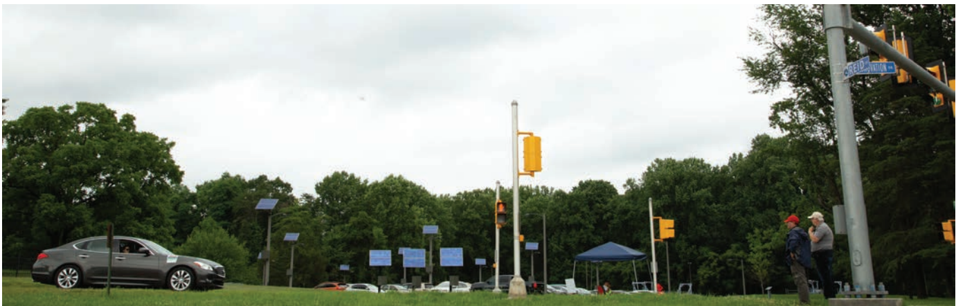
A THEA vehicle on a controlled test track at TFHRC approaches an intersection with a roadside unit. Photo: USDOT.
