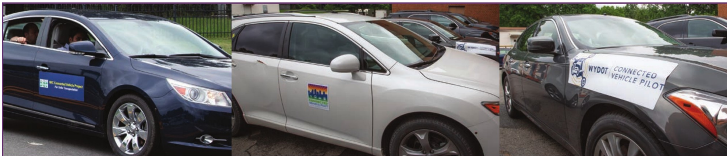
The USDOT Connected Vehicle Pilot Interoperability Test successfully demonstrated interactions among different sites' onboard units and among selected onboard and roadside units. Source: USDOT.
