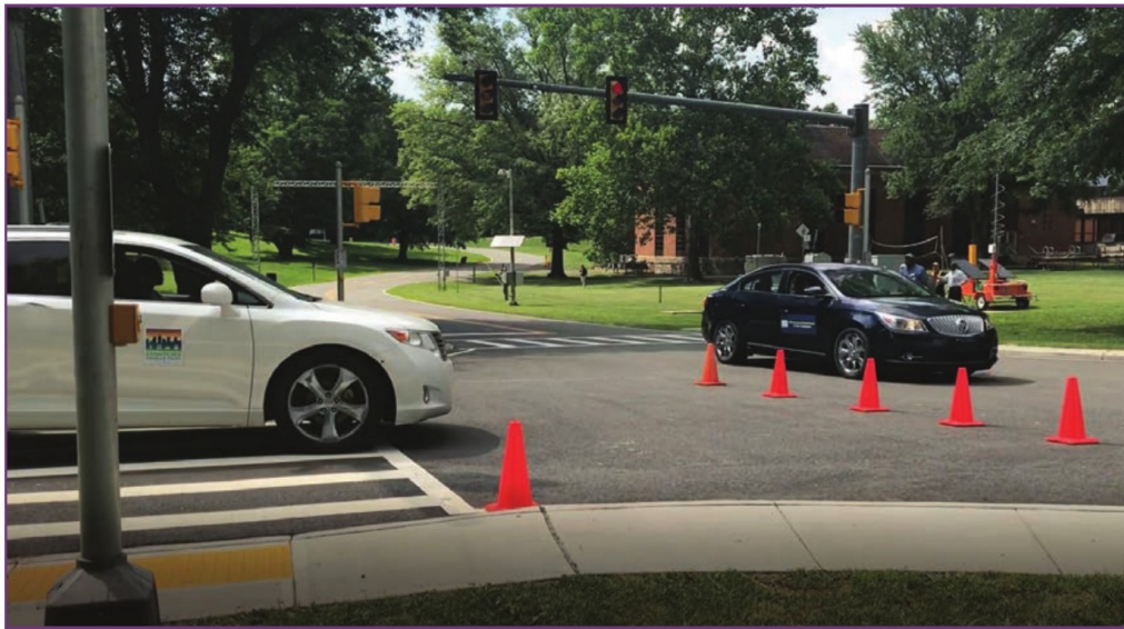
A vehicle from Tampa (white car) waits as it receives an intersection movement assist warning from a New York City vehicle (black car) during the interoperability test. Source: USDOT.
