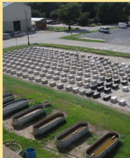
Outdoor exposure sites for durability testing at the University of Texas at Austin. © Racheal Lute.
