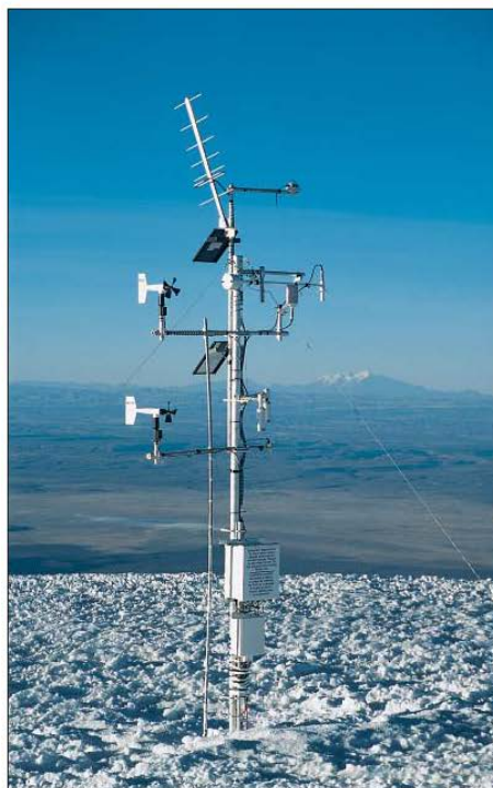
A GOES satellite system transmits data from a remote weather station in Nevado Sajama, Bolivia, to climate researchers in the United States.
