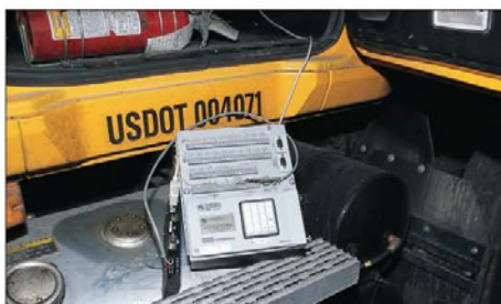
The SDM-CAN (left of CR5000) allows a vehicle's on-board diagnostic system to output standardized data streams that are synchronized with other measurements and stored in the CR5000.
