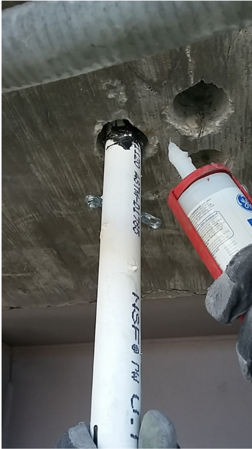
Figure 3.9 Tube with the thermocouples inside, with the cable tips protruding
