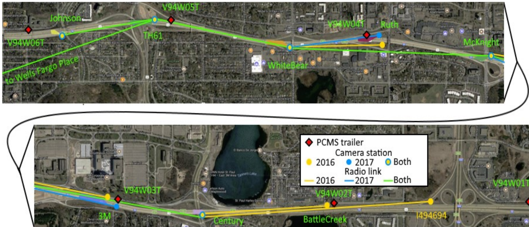
Figure 1.2 Work zone with PCMS trailers, camera stations, and radio links
