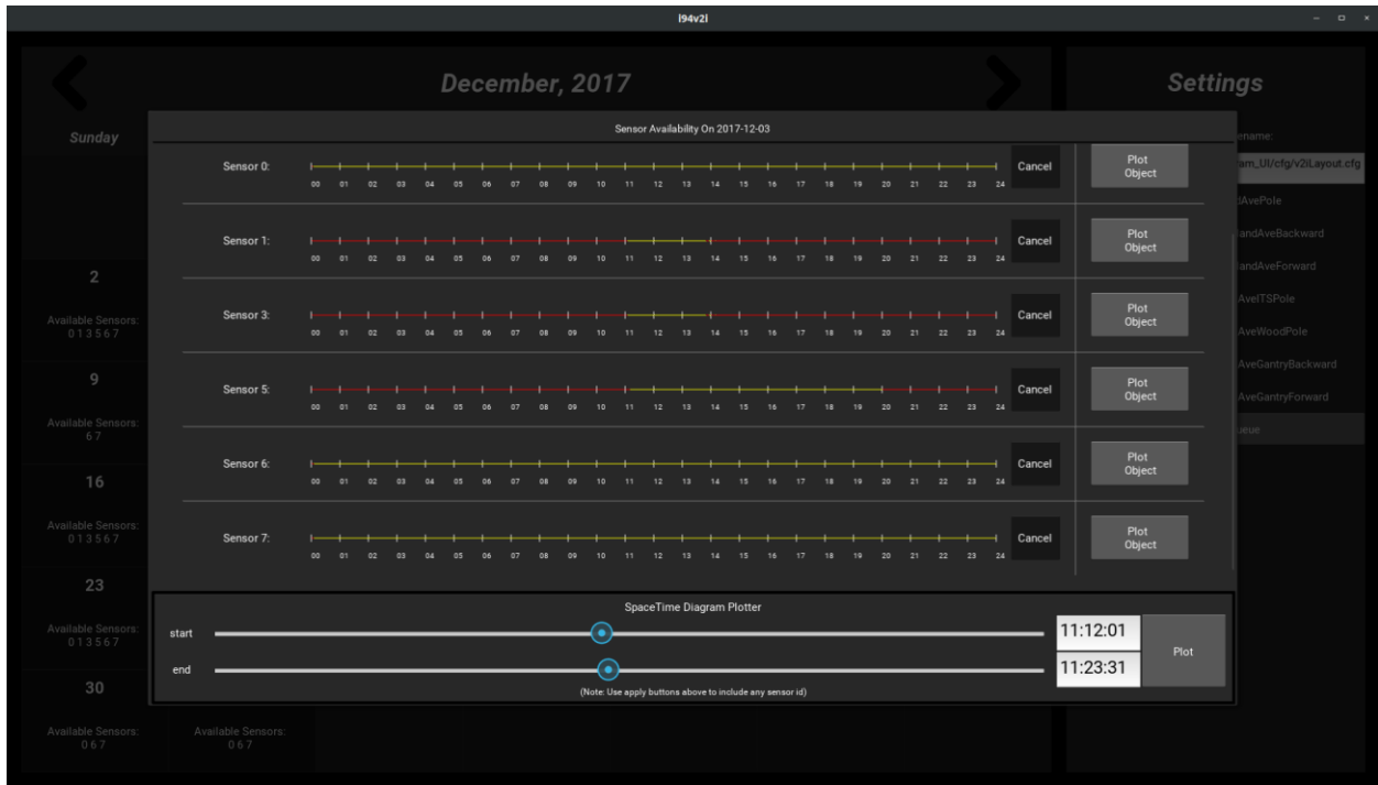
Figure C.4 Sensors have been selected and start and end times set by the user.
