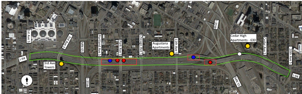
Figure 2.2 New testbed site showing radar sites (red dots), Wavetronix sites (blue dots), radar coverage (red outlines), rooftop stations (yellow dots), and a future MnDOT station (white dot).
