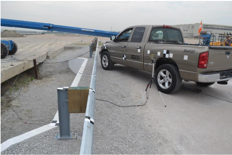
Figure 66. Impact Location, Test No. MGSL-2
