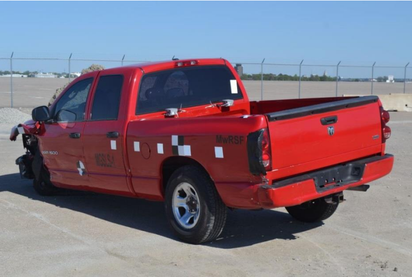
Figure 56. Vehicle Damage, Test No. MGSLS-1
