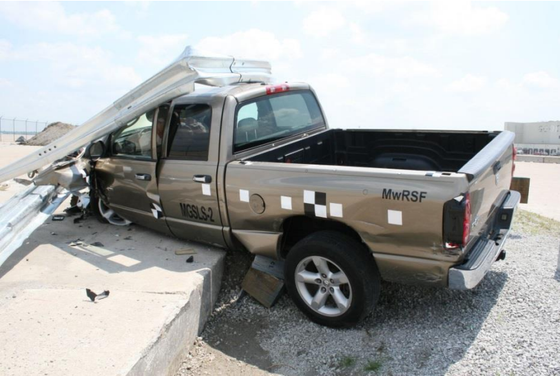
Figure 81. Vehicle Damage, Test No. MGSL-2
