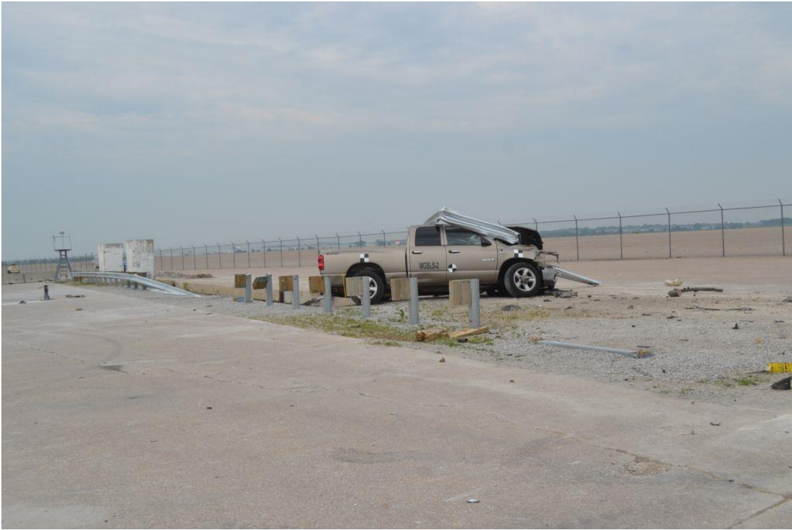
Figure 67. Vehicle Final Position and Trajectory Marks, Test No. MGSL-2
