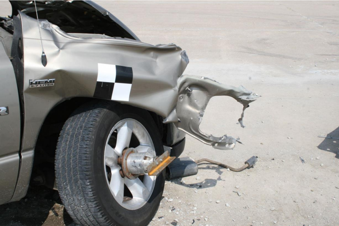
Figure 83. Vehicle Damage, Right Fender, Test No. MGSLS-2
