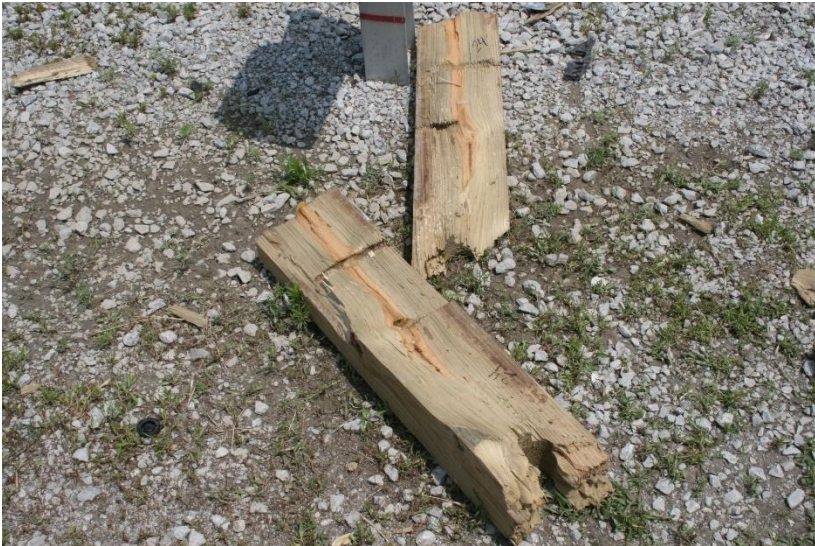
Figure 80. Downstream Anchorage Damage, Test No. MGSLS-2
