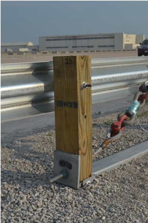
Figure 40. Test Installation Anchorage (Downstream), Test No. MGSL-2
