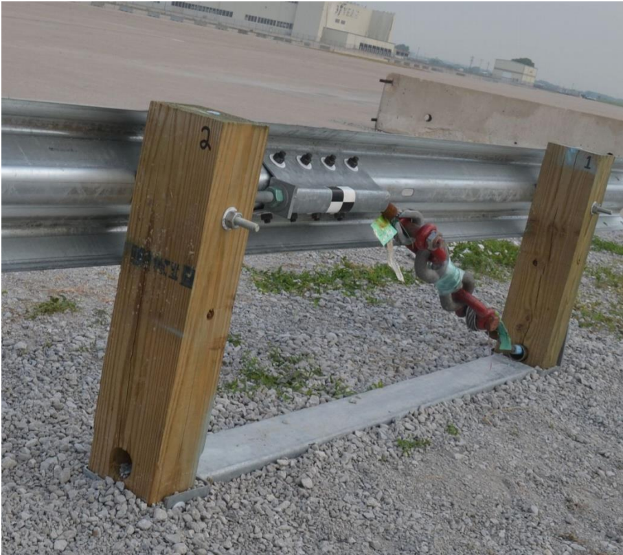
Figure 41. Test Installation Anchorage (Upstream), Test No. MGSLs-2
