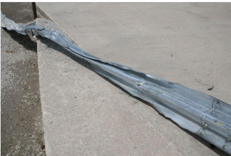
Figure 77. Damage to Rail Between Post Nos. 17 through 19, Test No. MGSLs-2
