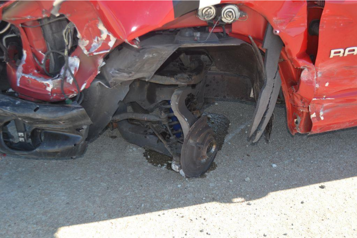
Figure 57. Vehicle Damage, Left Fender, Test No. MGSL-1
