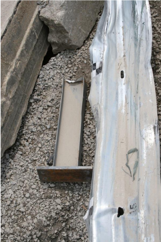
Figure 73. Damage at Post No. 14, Test No. MGSLs-2
