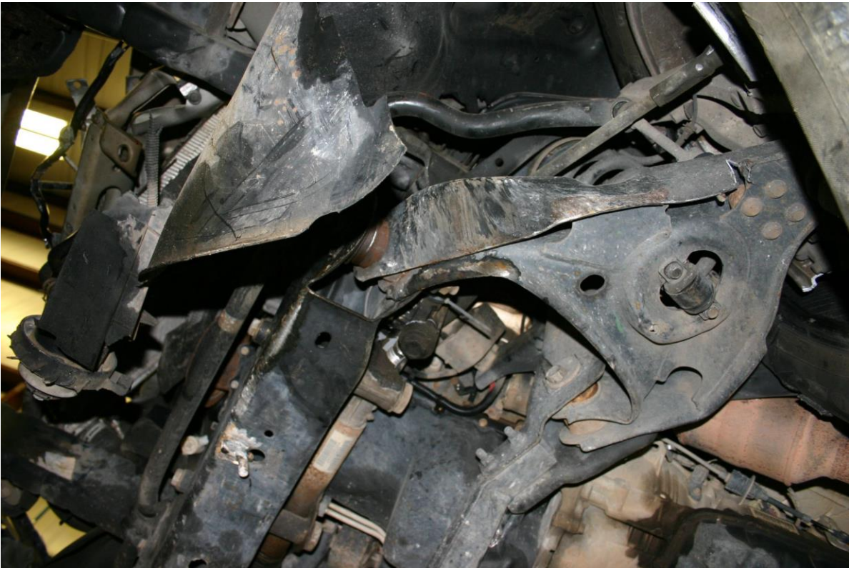
Figure 85. Vehicle Undercarriage Damage, Test No. MGSLs-2
