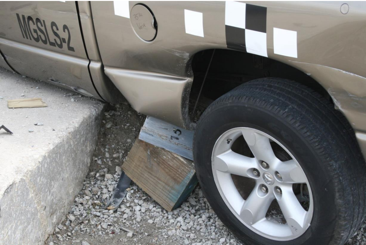
Figure 74. Damage at Post No. 15, Test No. MGSL-2
