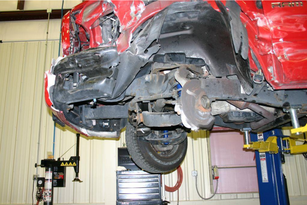
Figure 58. Vehicle Undercarriage Damage, Test No. MGSLs-1
