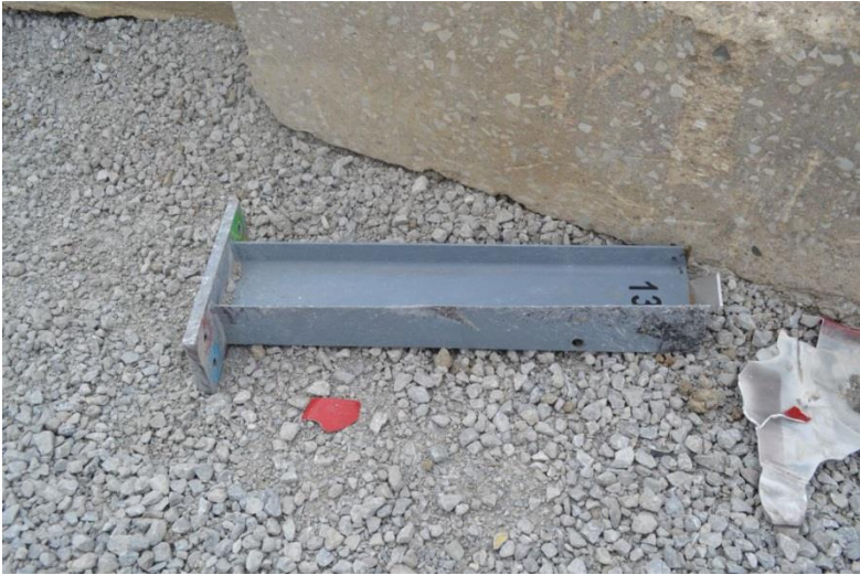
Figure 52. Damage at Post No. 13, Test No. MGSLs-1
