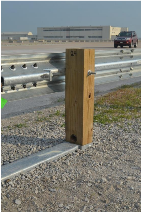
Figure 40. Test Installation Anchorage (Downstream), Test No. MGSL-2
