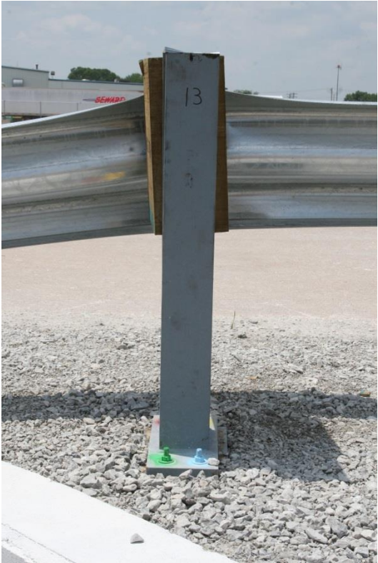
Figure 71. Damage at Post No. 13, Test No. MGSLS-2
