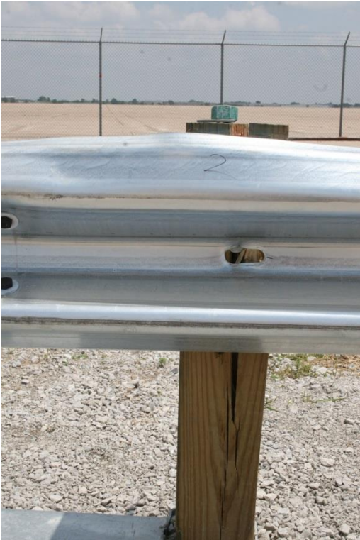
Figure 69. Upstream End Anchor Damage, Test No. MGSLS-2
