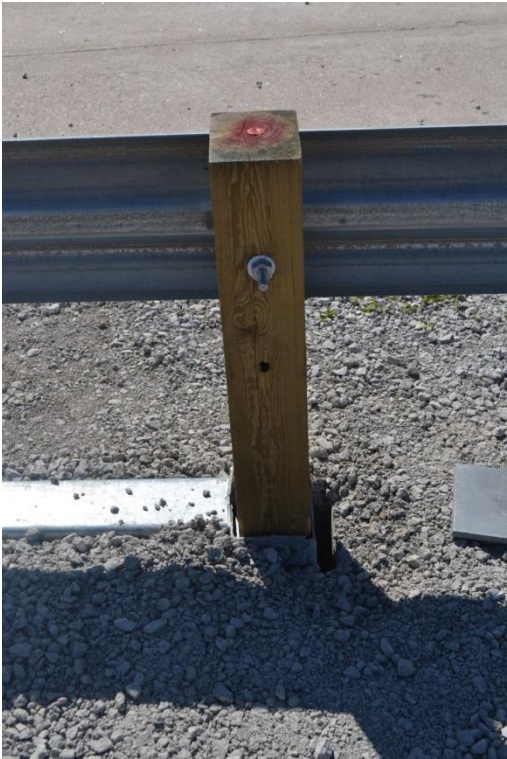
Figure 49. Upstream End Anchor Damage, Test No. MGSLS-1
