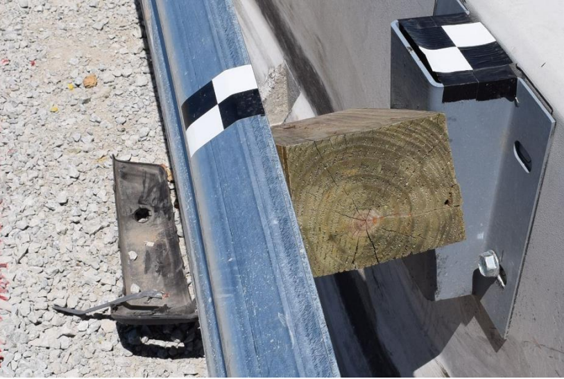
Figure 89. System Damage at the Transition, Test No. MGSPCB-2
