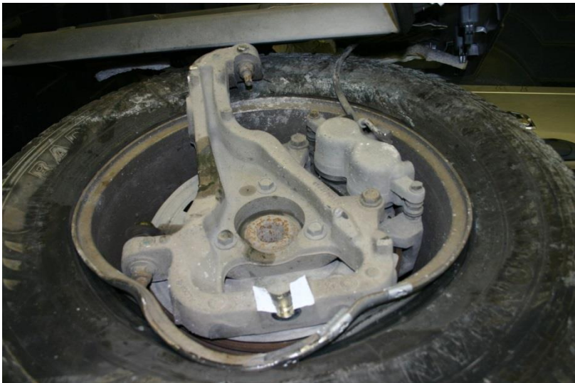
Figure 73. Undercarriage Damage, Test No. MGSPCB-1
