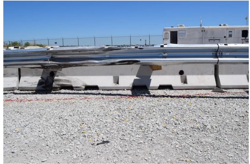
Figure 86. System Damage Between the End Shoe and Post No. 18, Test No. MGSPCB-2
