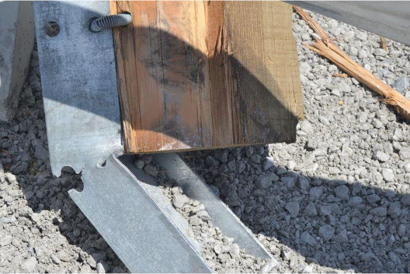
Figure 68. Post Nos. 16 and 17 Damage, Test No. MGSPCB-1
