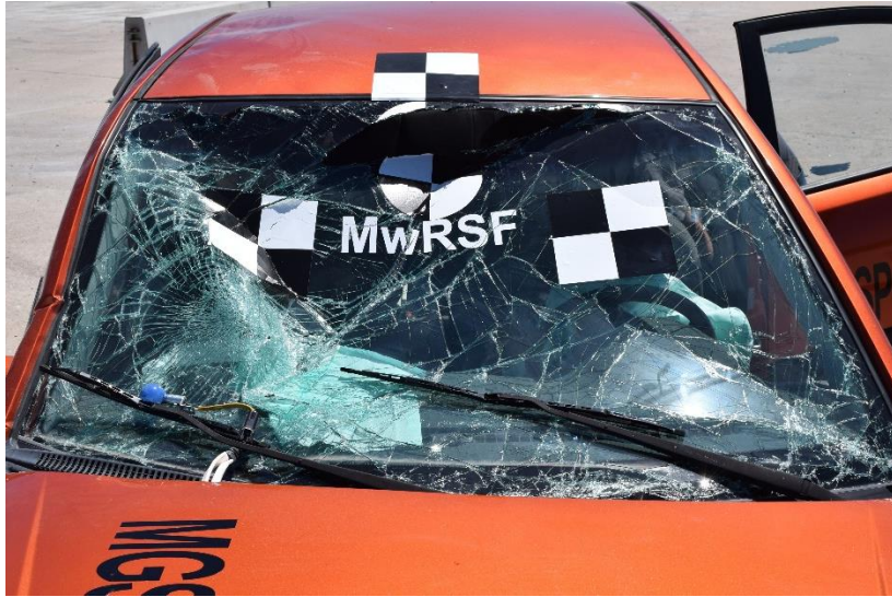
Figure 91. Vehicle's Windshield Damage, Test No. MGSPCB-2
