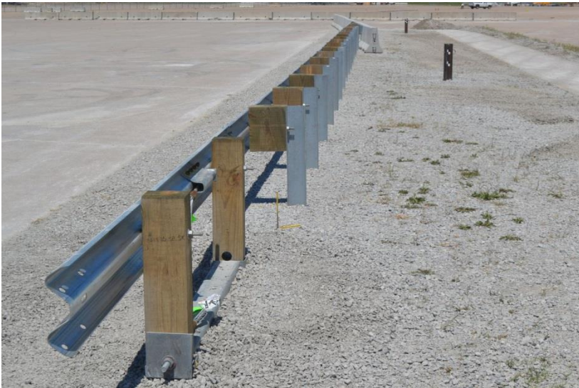
Figure 55. Test Installation, Test No. MGSPCB-1
