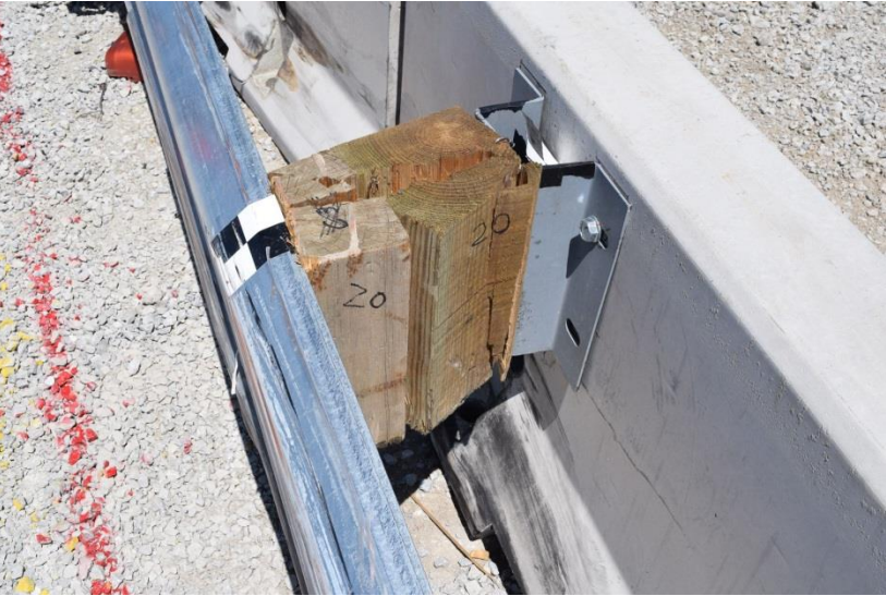
Figure 87. System Damage at the Transition, Test No. MGSPCB-2
