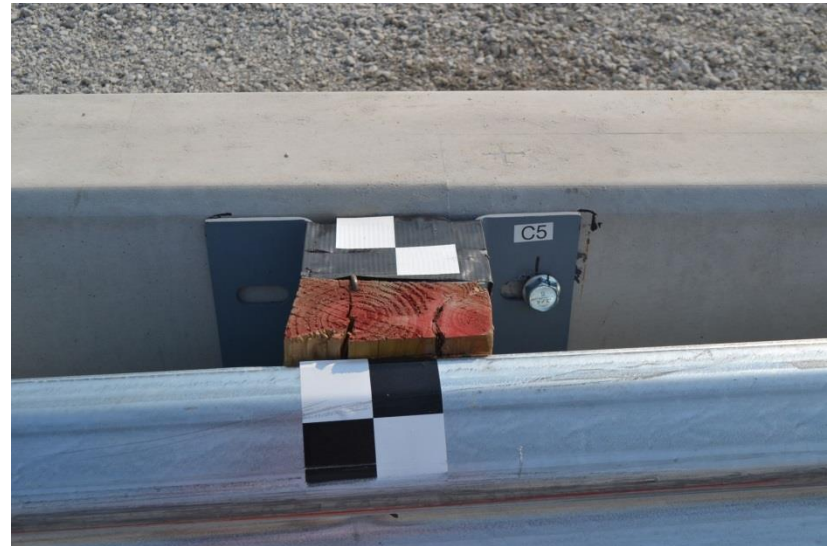
Figure 106. Rail and Blockout Damage Between End Shoe and Blockout C3, Test No. MGSPCB-3
