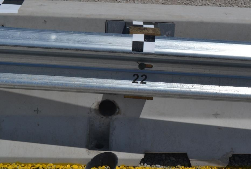
Figure 70. Damage at Non-Post Locations Nos. 30 through 23, Test No. MGSPCB-1
