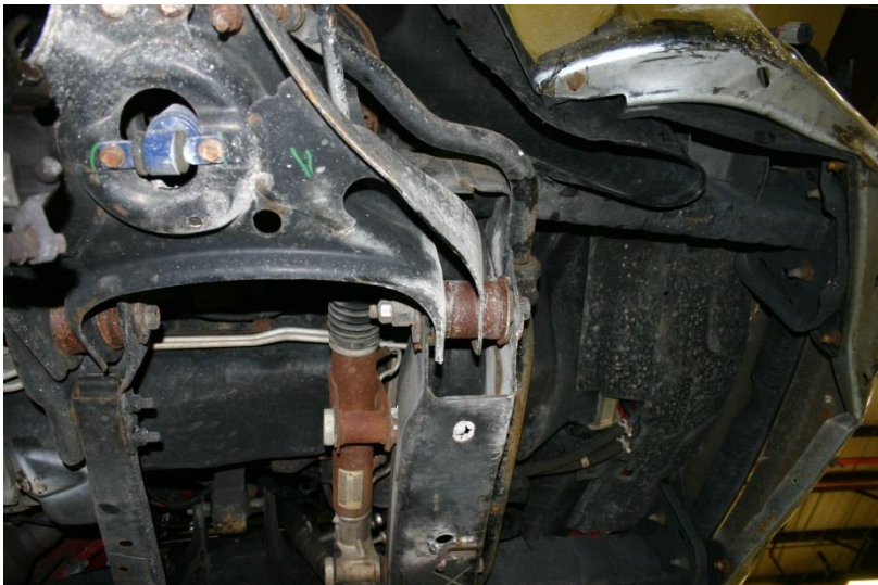
Figure 109. Undercarriage Damage, Test No. MGSPCB-3
