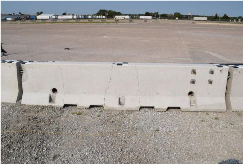
Figure 105. Backside Concrete Barrier Damage Between Concrete Barrier Nos. 7 and 8, Test No. MGSPCB-3
