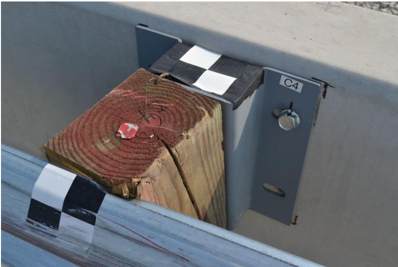
Figure 106. Rail and Blockout Damage Between End Shoe and Blockout C3, Test No. MGSPCB-3
