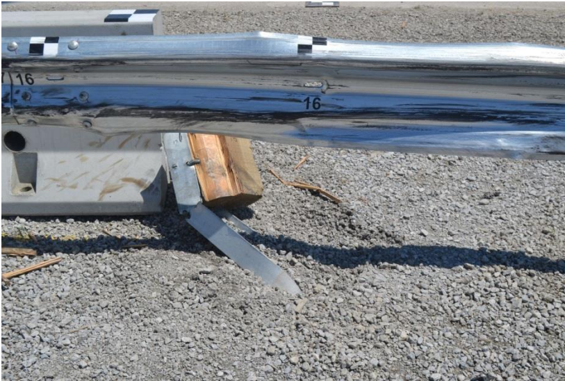
Figure 67. System Damage Between Post Nos. 14 and 18, Test No. MGSPCB-1
