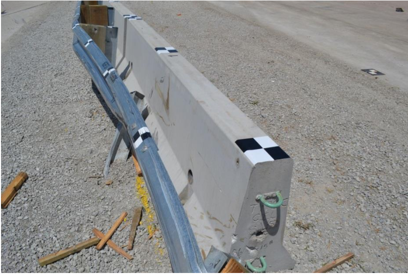
Figure 69. Transition Damage, Test No. MGSPCB-1
