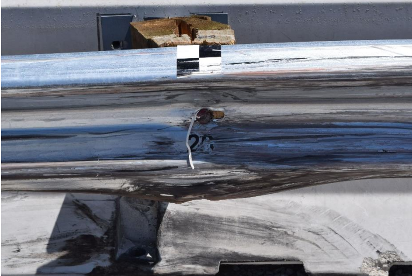
Figure 88. System Damage at the Transition, Test No. MGSPCB-2
