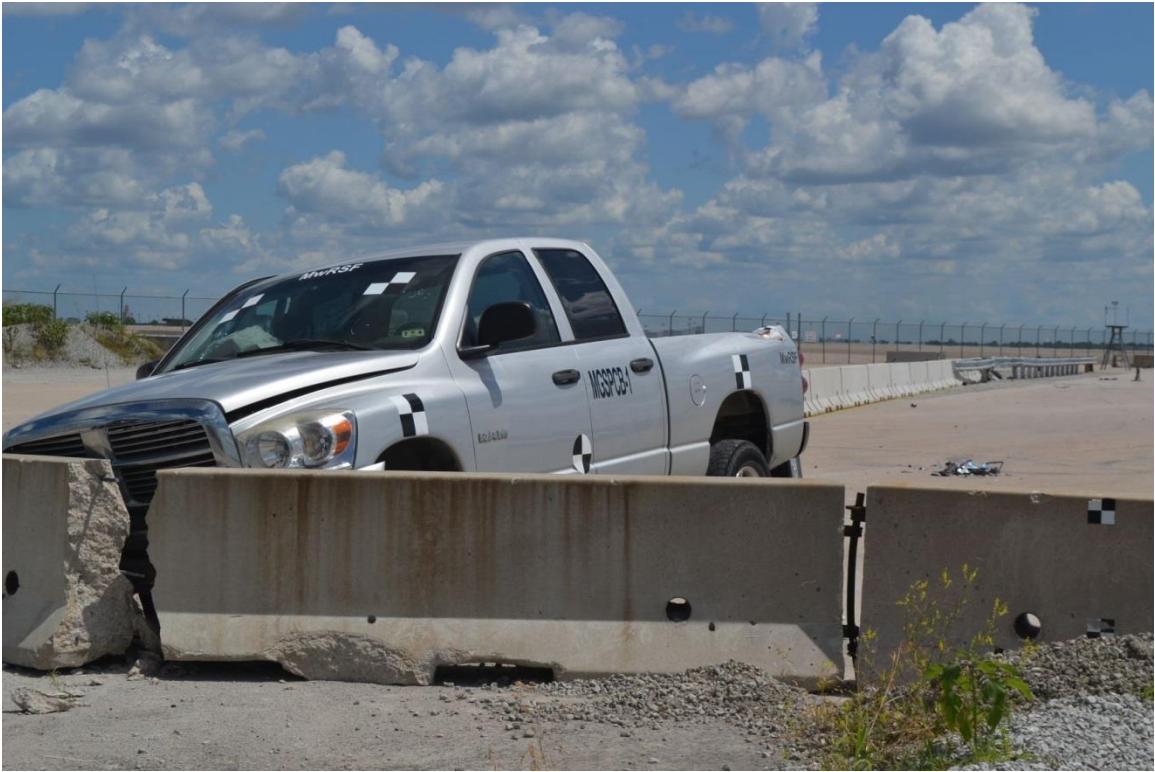
Figure 64. Vehicle Final Position, Test No. MGSPCB-1
