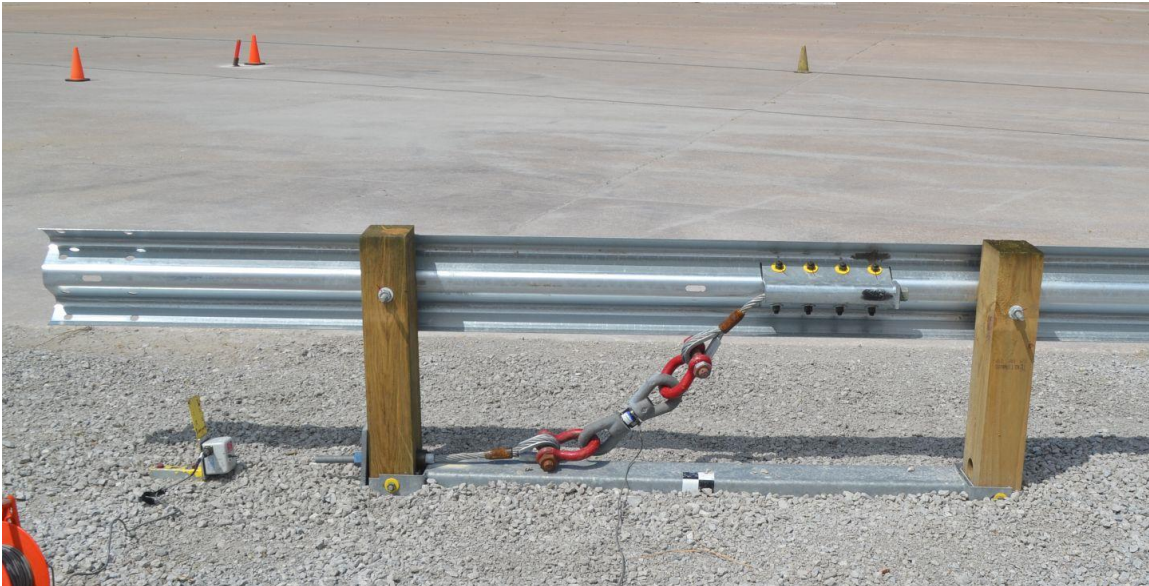
Figure 15. Location of Load Cells and String Potentiometers
