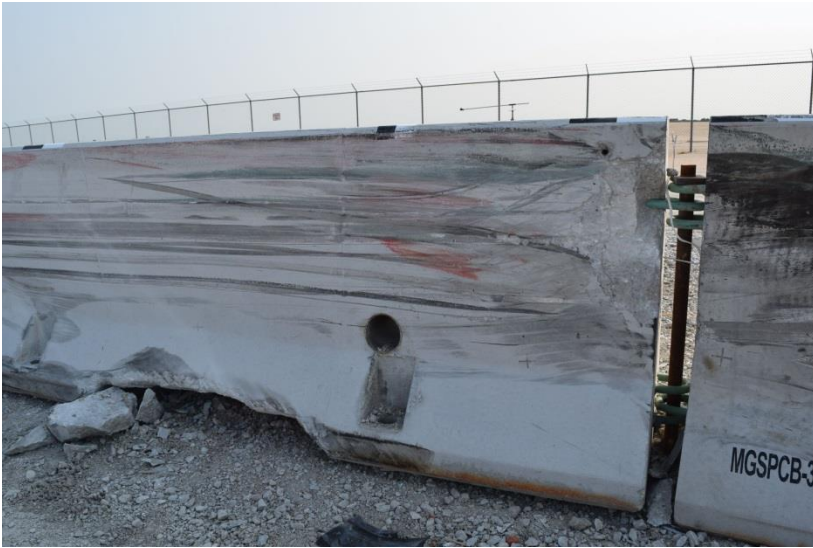
Figure 104. System Damage Between End Shoe and Concrete Barrier No. 7, Test No. MGSPCB-3
