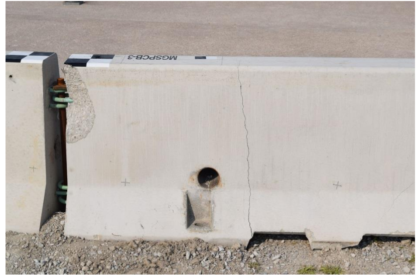
Figure 105. Backside Concrete Barrier Damage Between Concrete Barrier Nos. 7 and 8, Test No. MGSPCB-3
