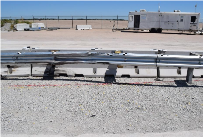
Figure 86. System Damage Between the End Shoe and Post No. 18, Test No. MGSPCB-2
