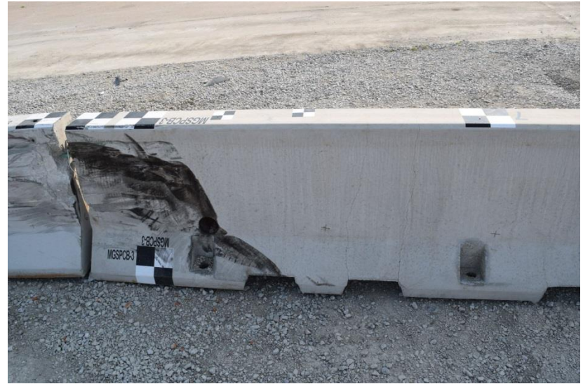
Figure 104. System Damage Between End Shoe and Concrete Barrier No. 7, Test No. MGSPCB-3
