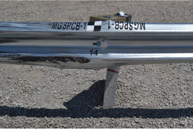
Figure 66. System Damage Between Post Nos. 12 and 15, Test No. MGSPCB-1
