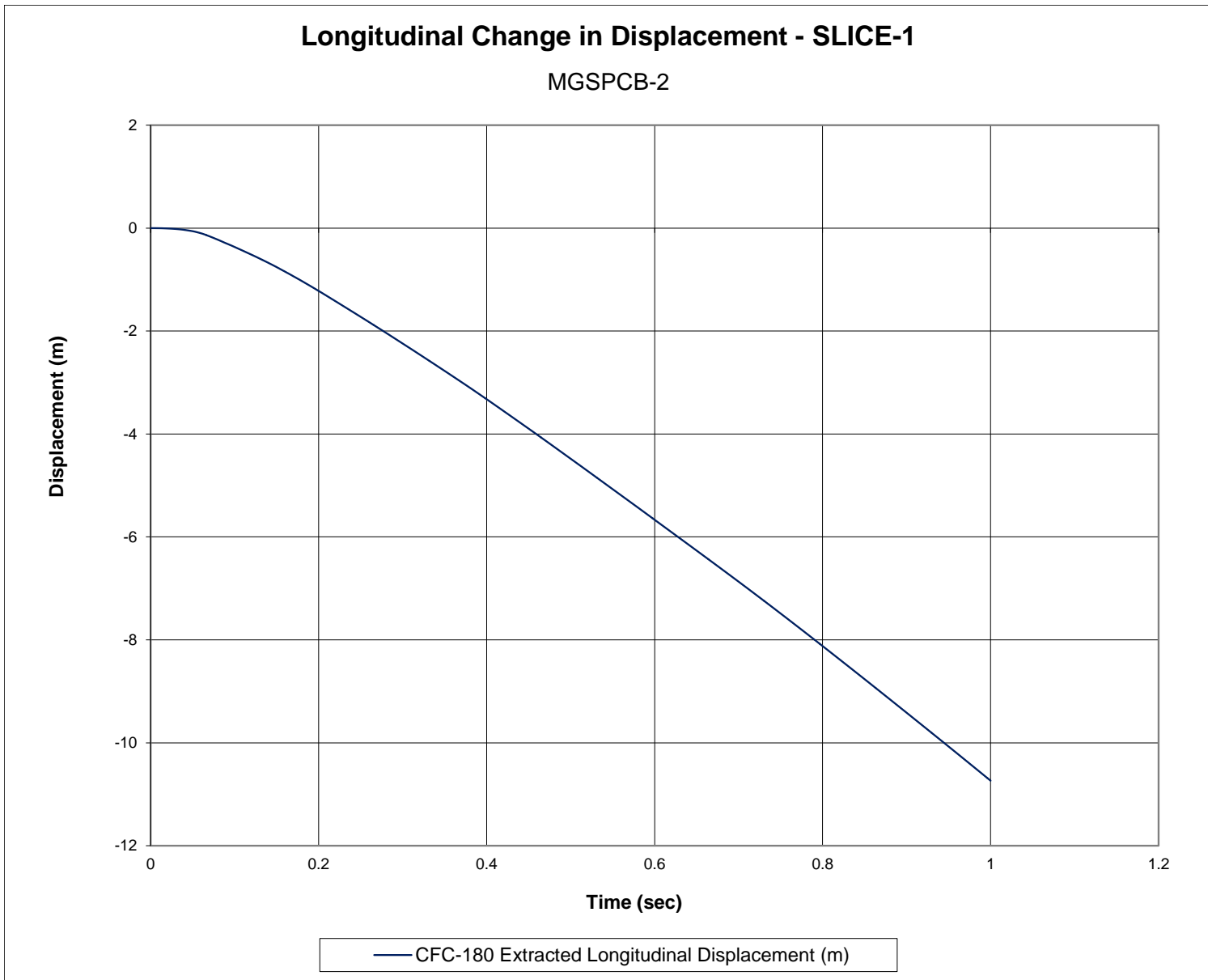
Figure G-3. Longitudinal Occupant Displacement (SLICE-1), Test No. MGSPCB-2
