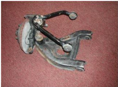
Figure 2. C2500 Main Suspension Components
