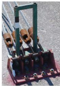
Figure 34. Cable Anchor Bracket and Finite Element Model
