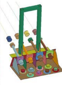
Figure 34. Cable Anchor Bracket and Finite Element Model
