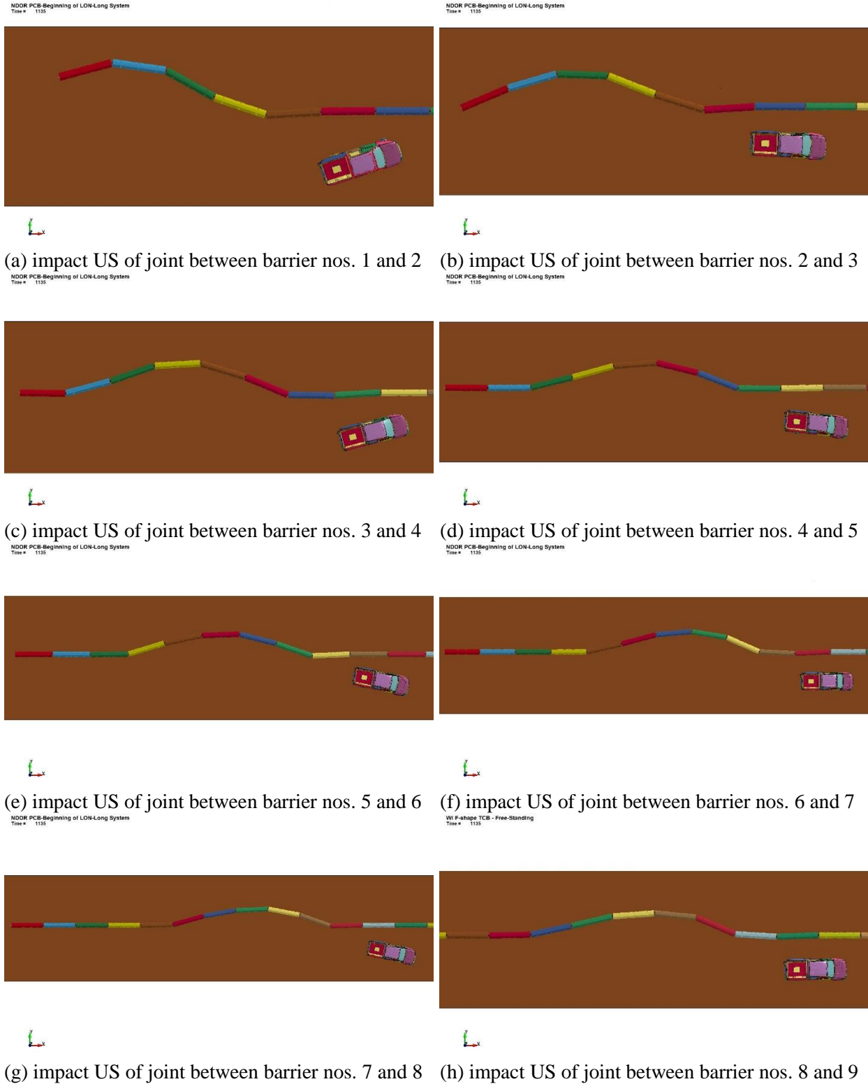
Figure 16. Simulation of Beginning of LON for 16-Barrier F-Shape PCB System, Overhead View, t=1.100 sec
