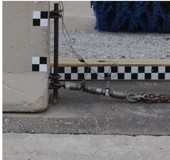
Figure 2. Load Cell Arrangement, Test No. TCBFA-1
