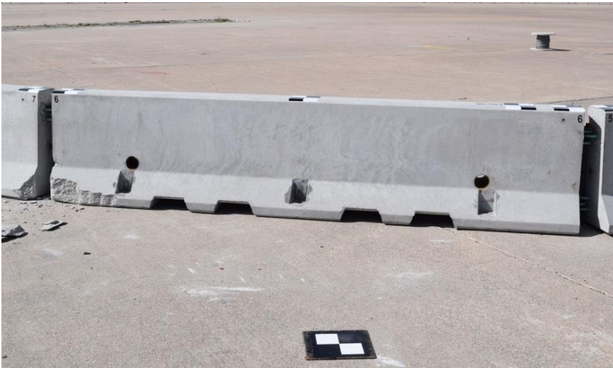
Figure 95. Barrier No. 6 Damage, Test No. NELON-2
