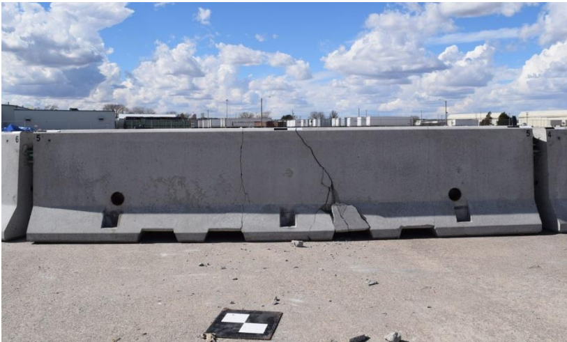
Figure 94. Barrier No. 5 Damage, Test No. NELON-2
