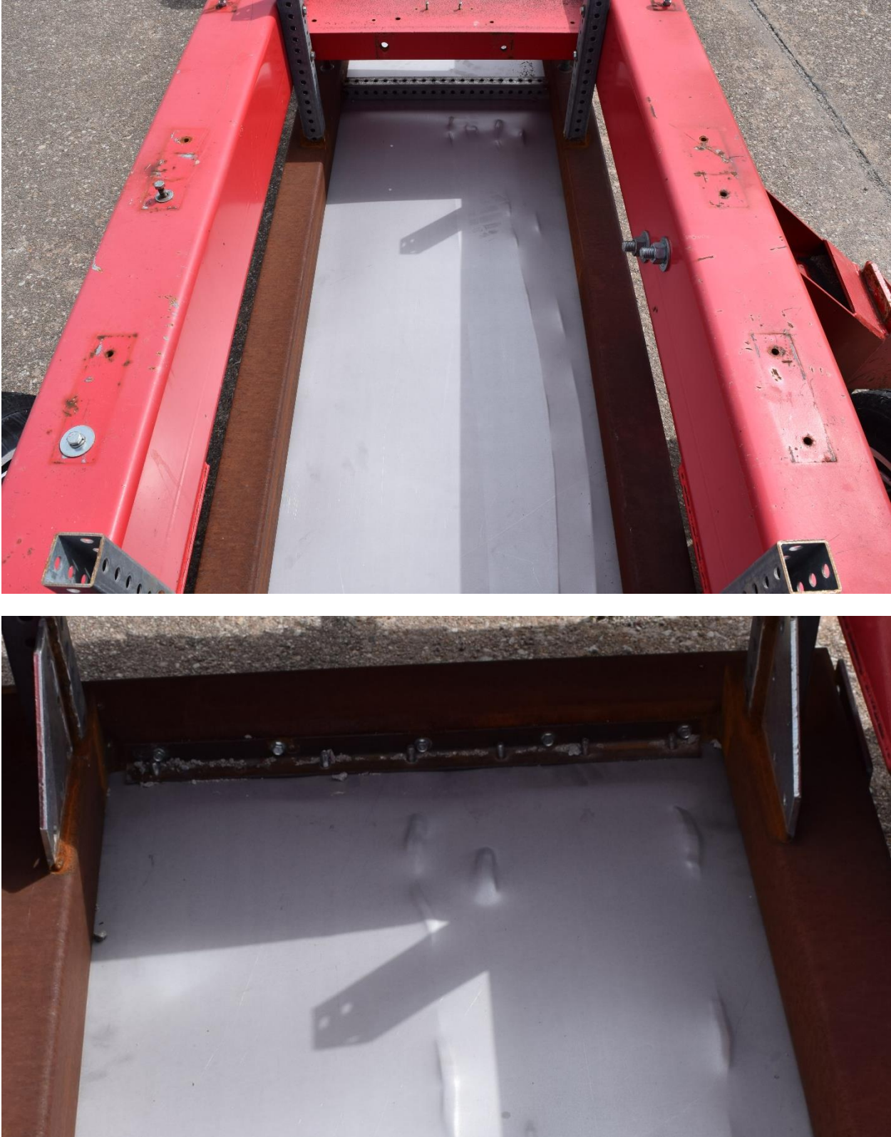
Figure 32. Simulated Floor Pan Damage, Test No. MWFPF-24
