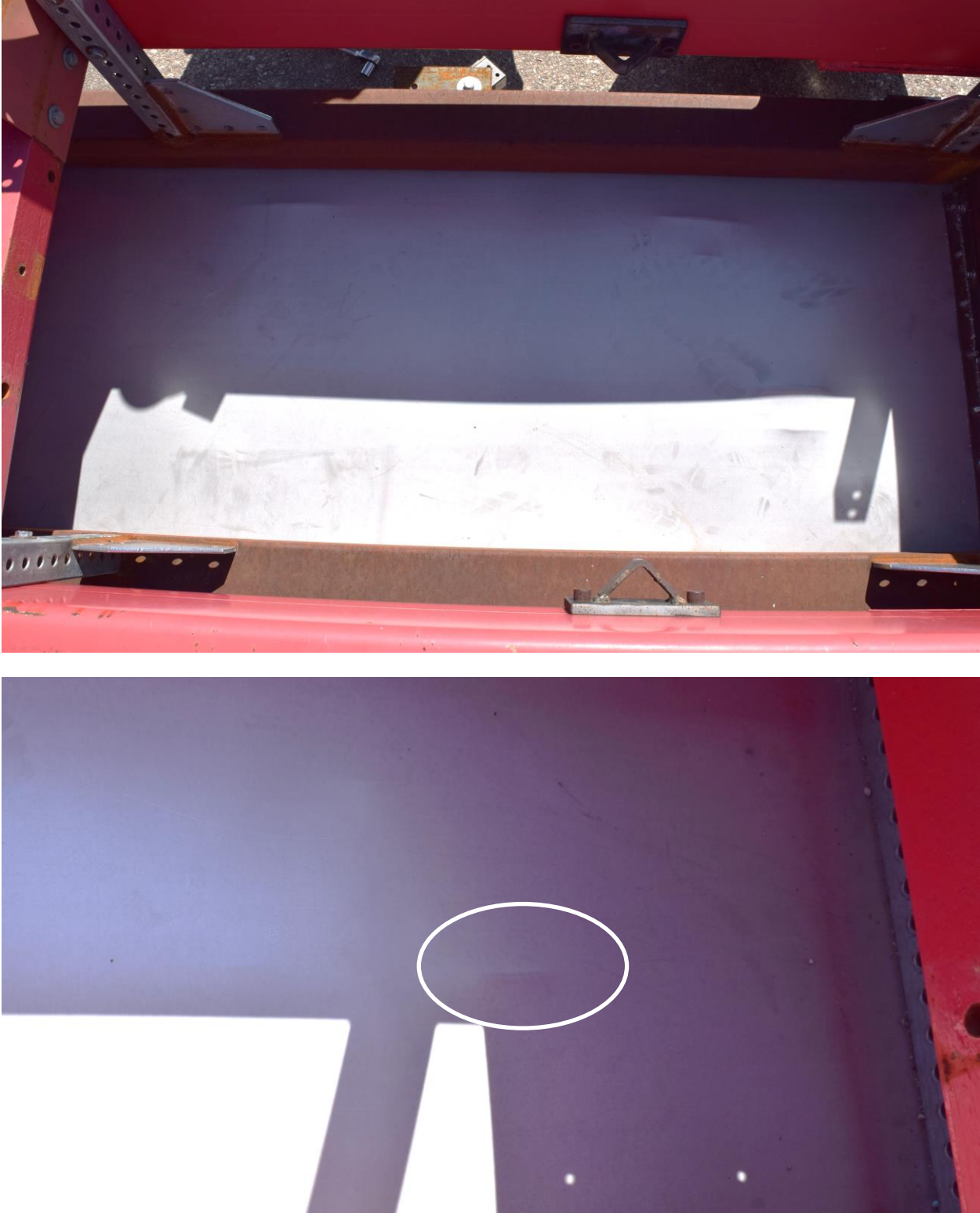
Figure 35. Simulated Floor Pan Damage, Test No. MWFPF-25
