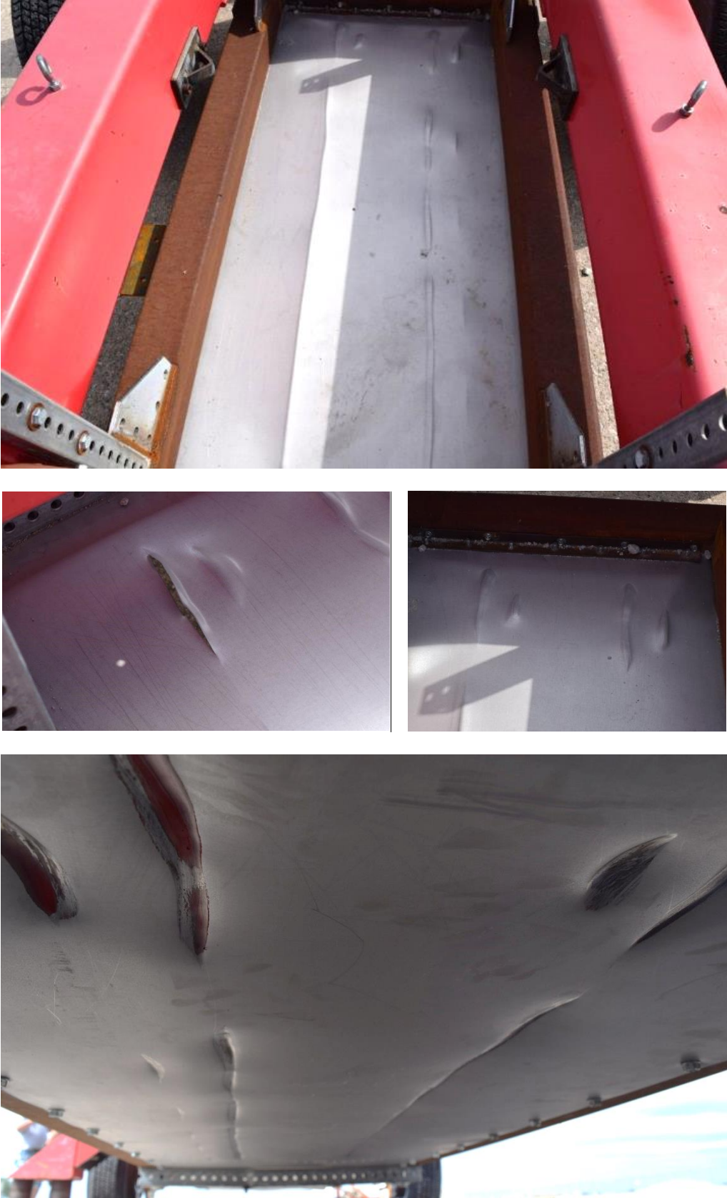
Figure 29. Simulated Floor Pan Damage, Test No. MWFPF-23
