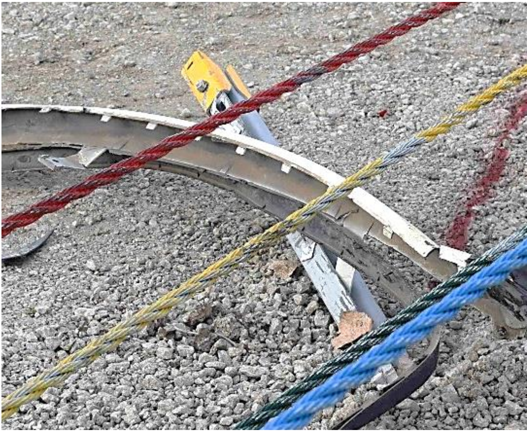
Figure 65. Post No. 33 Damage, Test No. MWP-9
