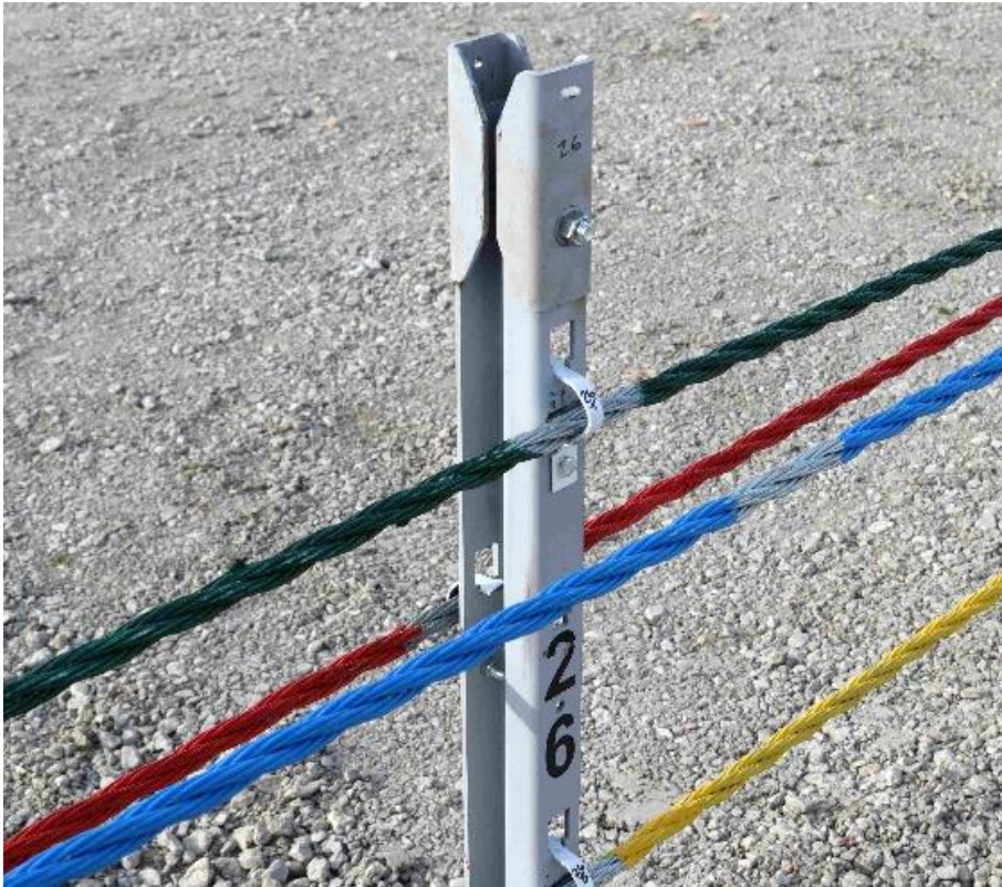
Figure 58. Post No. 26 Damage, Test No. MWP-9
