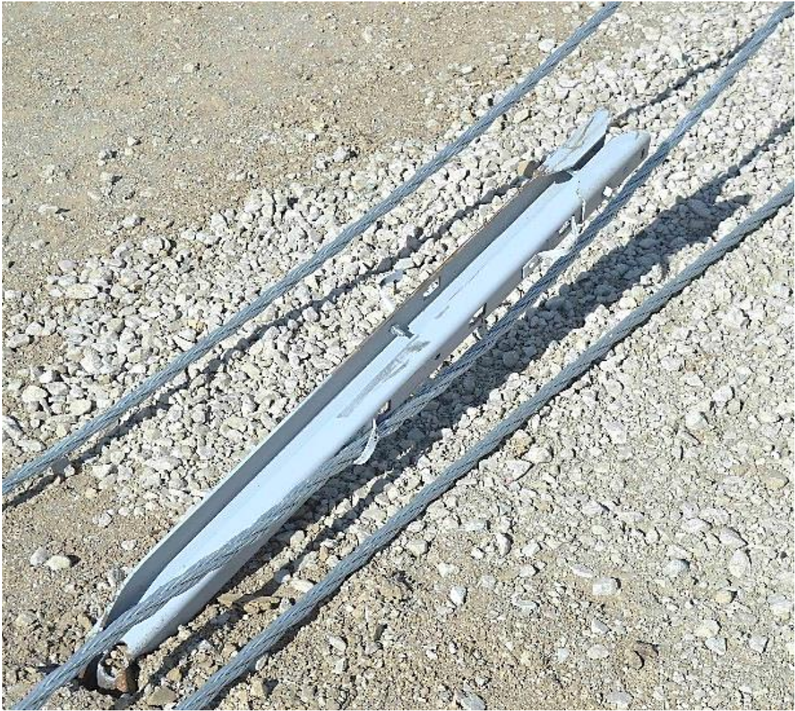
Figure 81. Post No. 49 Damage, Test No. MWP-9
