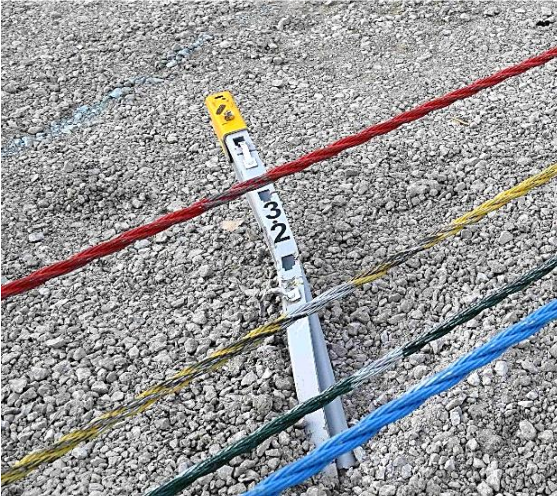
Figure 64. Post No. 32 Damage, Test No. MWP-9
