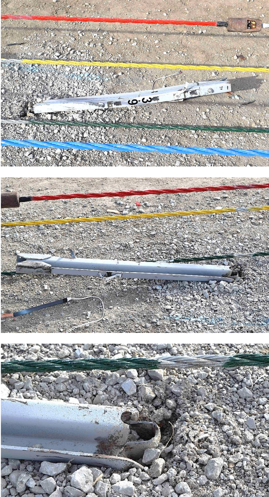
Figure 71. Post No. 39 Damage, Test No. MWP-9
