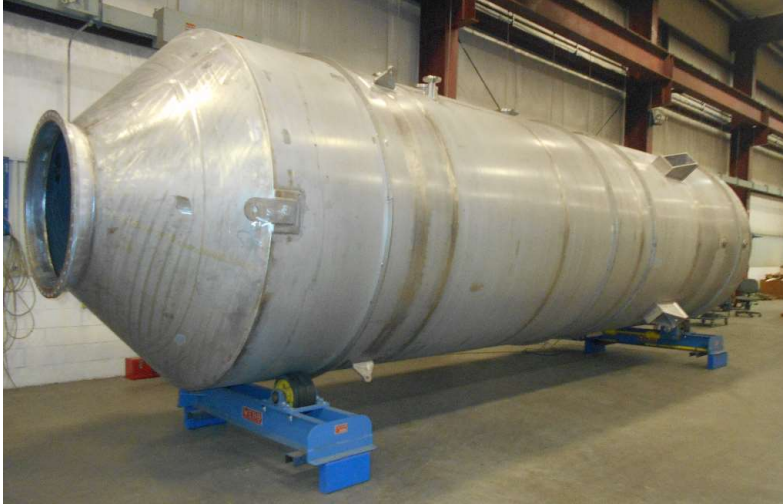
Scrubber vessel during fabrication
