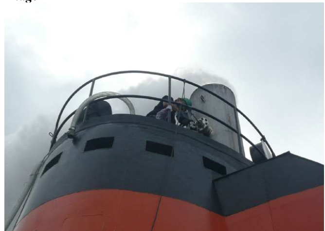
Sampling ports after Scrubber
