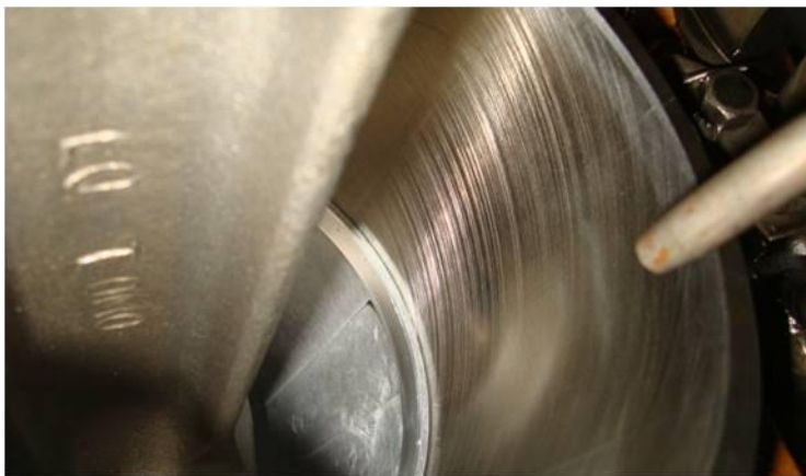
Figure 29. Cylinder Number 6 -Lower End Hone Marks
