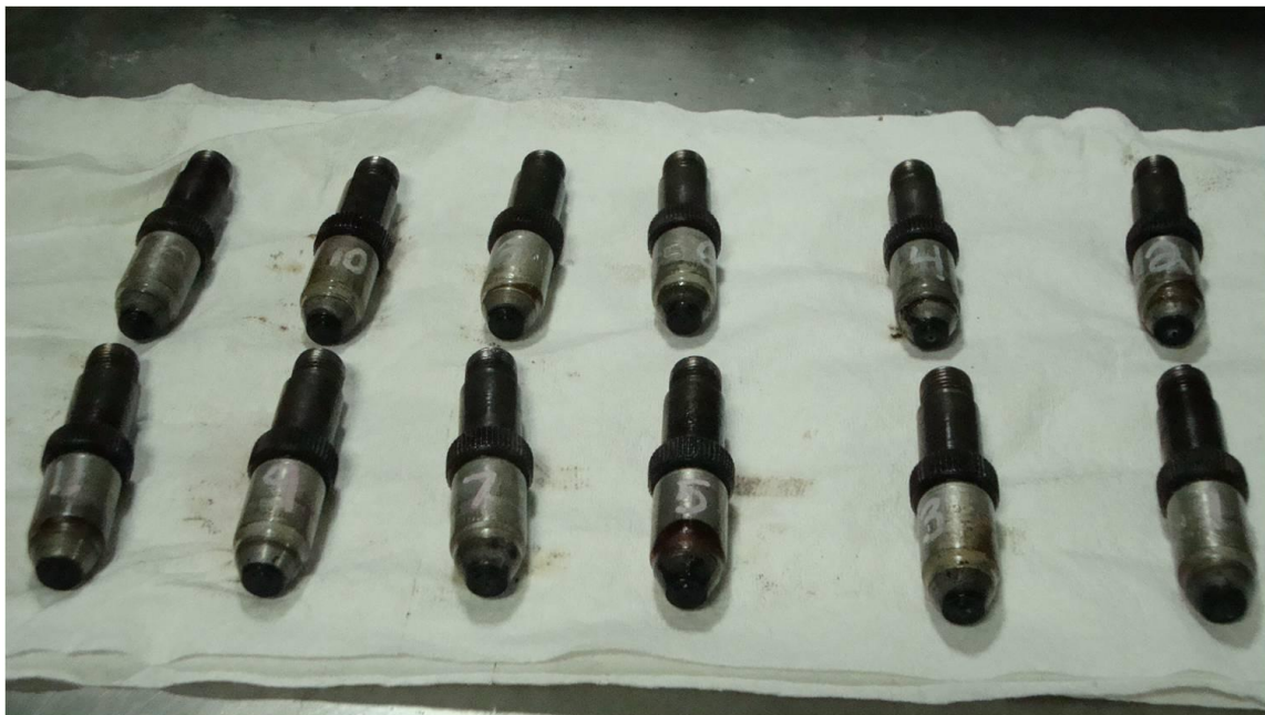
Figure 25. Post-Test Condition of Number 4 SSDG Nozzle Assemblies
