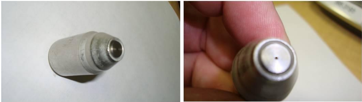
Figure 22. New Nozzle Tip
