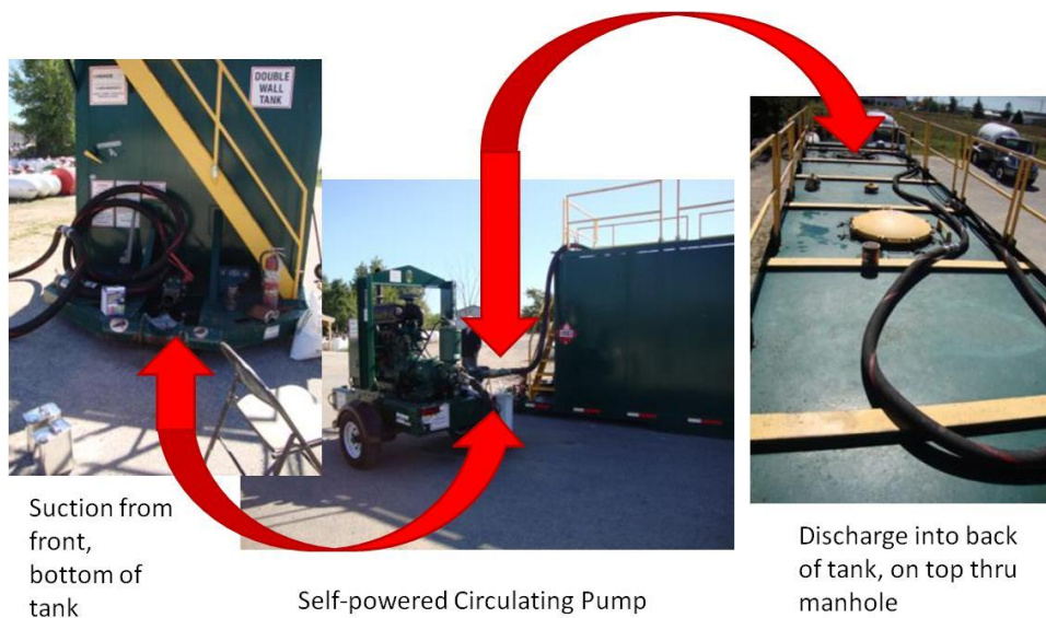
Figure 12. Fuel Blending Configuration at Fuel Provider Facility
