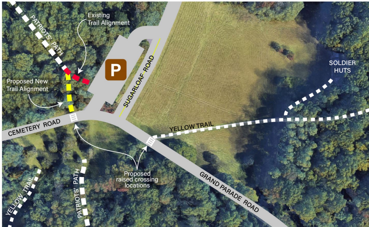
Figure 3-14: Detailed plan view of proposed raised crossing locations #8 and #9 and Patriots' Path trail realignment. Source: Volpe
