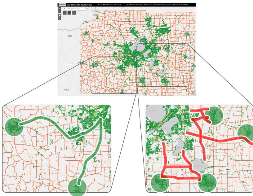
Figure 7: Screenshots of the bicycle LTS web map route finder show arterials with and without bicycle infrastructure improvements. The image on the lower left shows a section with a low-LTS connection, and the image on the lower right shows a high-LTS barrier. (Image courtesy of Madison Area Transportation Planning Board and the Volpe Center)
