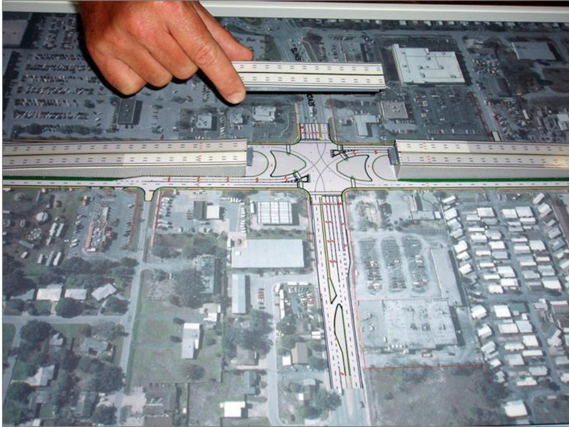
Figure 3. Advanced Visualization: 2-D Graphic with a 3-D Overlay Aerial photo and plan drawing with 3-D model components of proposed infrastructure. Source: FDOT.
