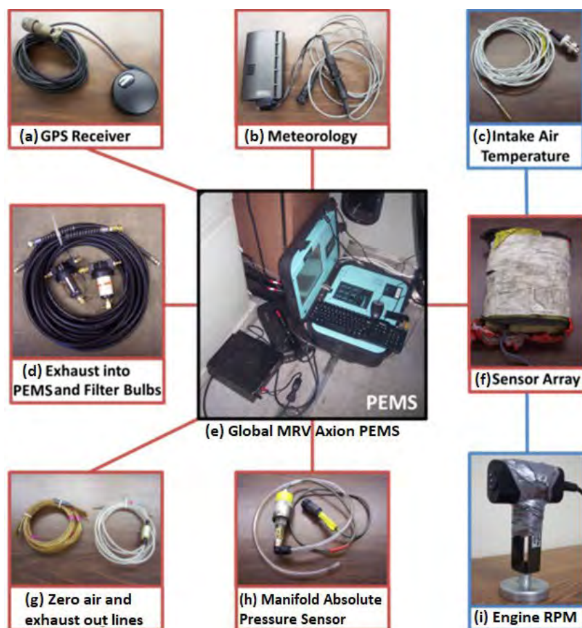
FIGURE 3-1. The GlobalMRV Axion PEMS and components: (a) GPS receiver; (b) Meteorology sensor; (c) Intake Air Temperature Sensor; (d) Exhaust sample lines; (e) Axion PEMS; (f) Engine sensor array; (g) Zero air and exhaust-out lines; (h) Manifold Absolute Pressure sensor; and (i) Engine RPM sensor
