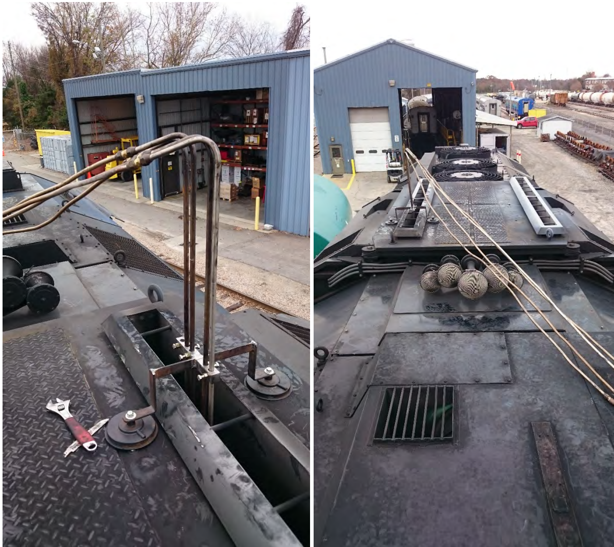
FIGURE D- 2. Sampling rake re-designed by NCDOT to collect exhaust sample from a single location
