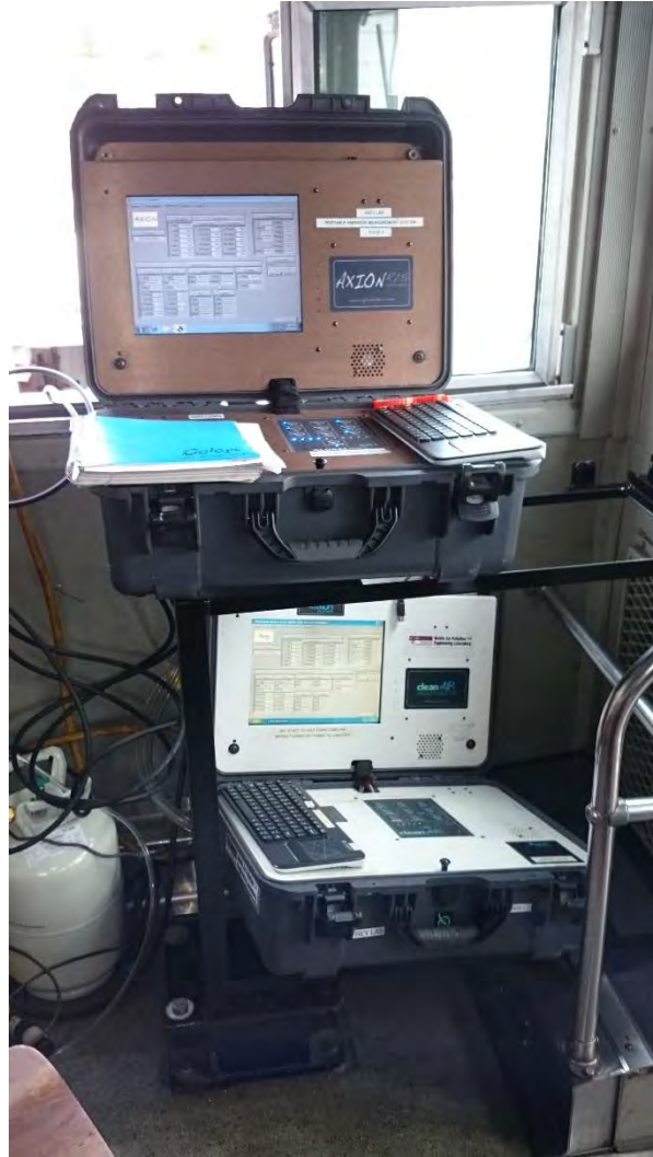
FIGURE D- 3. Rack designed by NCDOT to secure two Axion PEMS inside the locomotive cab
