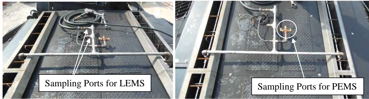
FIGURE 6-2. Installation of sampling rake at the outlets of BATS channels of the locomotive NC 1859.
