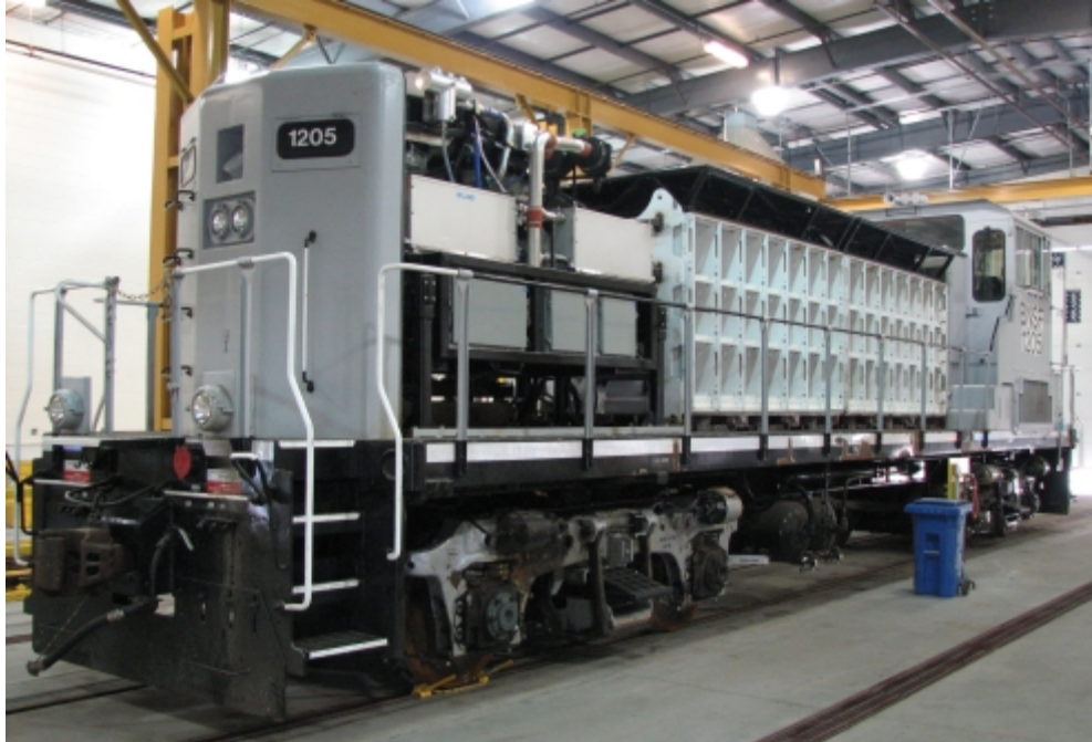
Figure 5. 1 st Photograph of the BNSF test platform for potential use in evaluating the prototype hybrid SOFC-GT system
