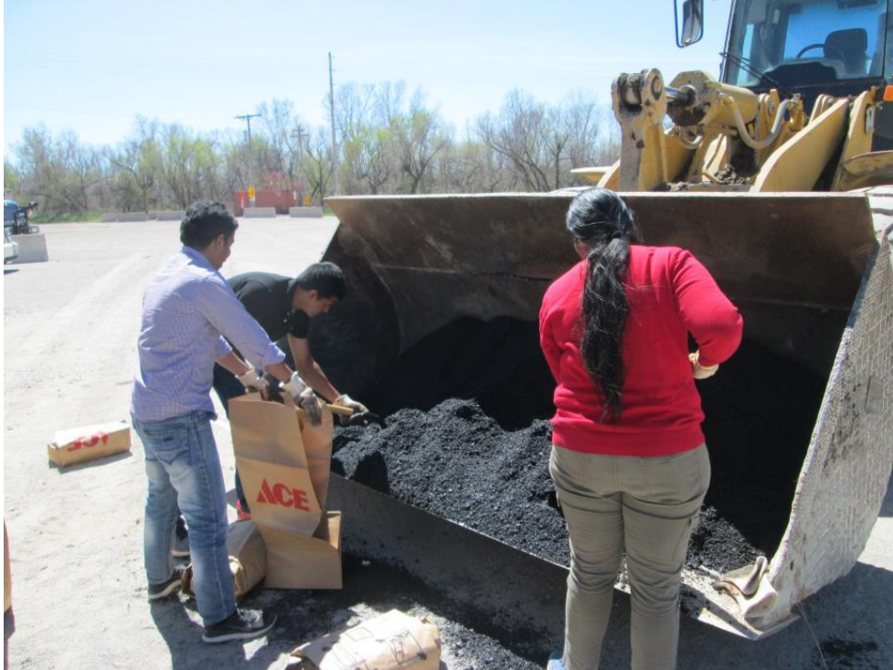
Figure 3.1 Collection of Asphalt Mix from Haskell Lemon Construction Co., Norman, OK
