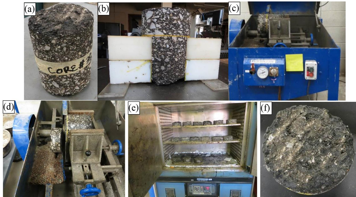
Figure 3.18 Photographic Views of the Procedure Followed for Preparing Field Cores for LISST Tests: (a) Typical Field Core; (b) Marking Sample; (c) Asphalt Saw; (d) Cut Sample, (e) Drying Samples in the Oven; and (f) Final Sample
