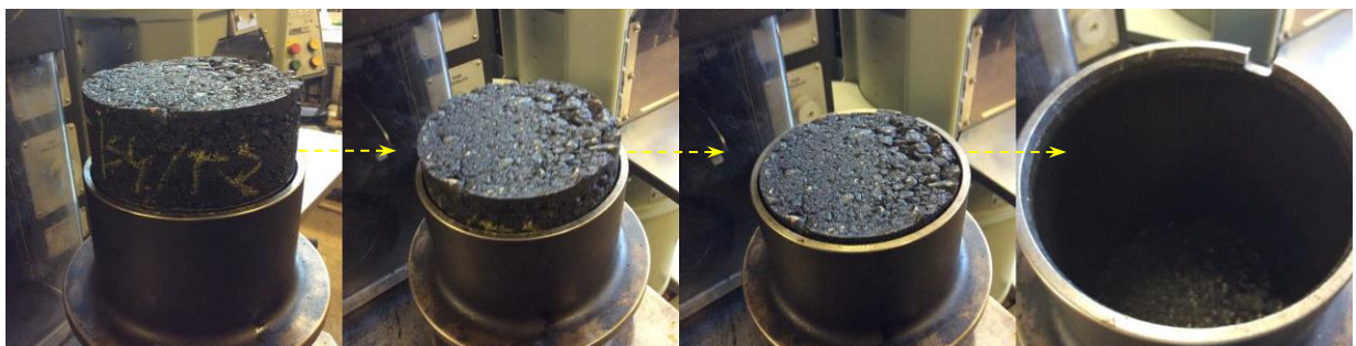
Figure 3.15 Sliding of Bottom Layer Sample into the SGC Mold Under Self-Weight
