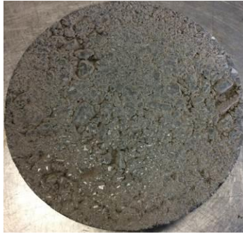
Figure 3.16 Asphalt Mix Sample after Polishing
