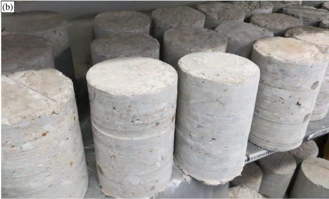
Figure 3.4 Field Cores of (a) Milled HMA; and (b) PCC
