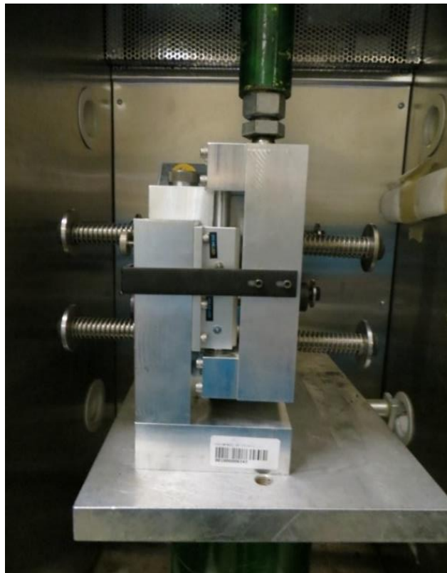
Figure 3.7 Louisiana Interlayer Shear Strength Test (LISST) Setup
