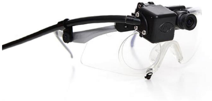
Figure 3.5 - UMass eye-tracking equipment [Source: https://imotions.com/ ]
