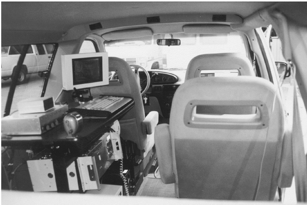
Figure 1. Example of Potential Monitor Mounting Bracket Problem
