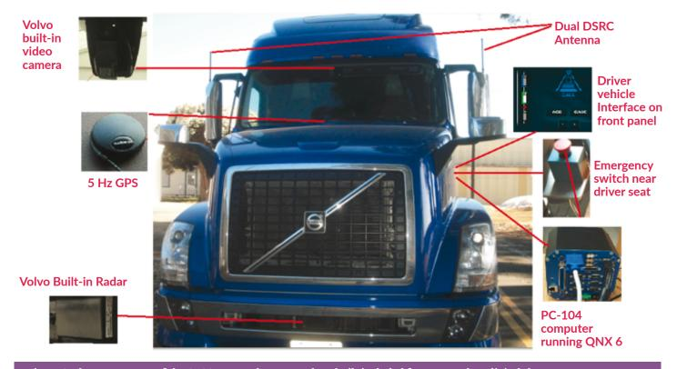
Figure 2. The components of the CACC system that researchers built included features such as digital short-range communications, a PC-104 computer, and a digital display. © California PATH.
