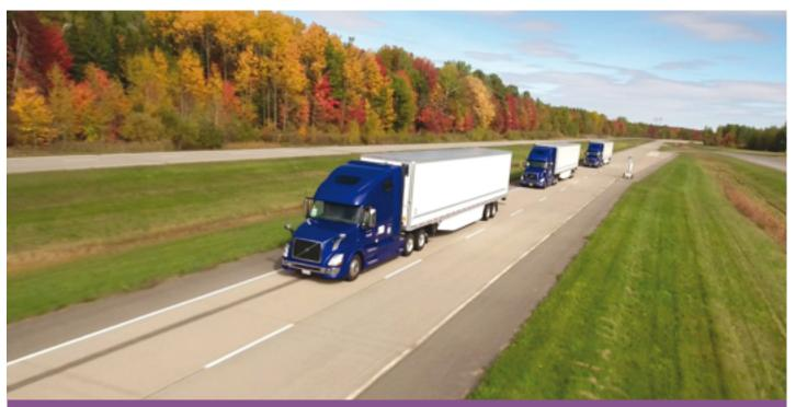
Figure 1. University of California-Berkeley researchers built a cooperative adaptive cruise control system into a platoon of three long-haul trucks to test the technology's potential to improve traffic flow, save fuel, and curtail emissions. © Transport Canada
