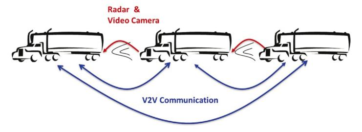
Figure 3. Trucks with CACC systems use radar and video cameras to "see" and vehicle-to-vehicle communication to "talk" to each other so they can maintain designated time gaps. © California PATH.
