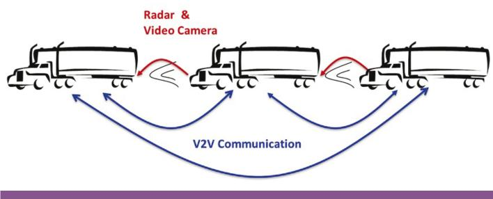
Figure 3. Trucks with CACC systems use radar and video cameras to "see" and vehicle-to-vehicle communication to "talk" to each other so they can maintain designated time gaps. © California PATH.
