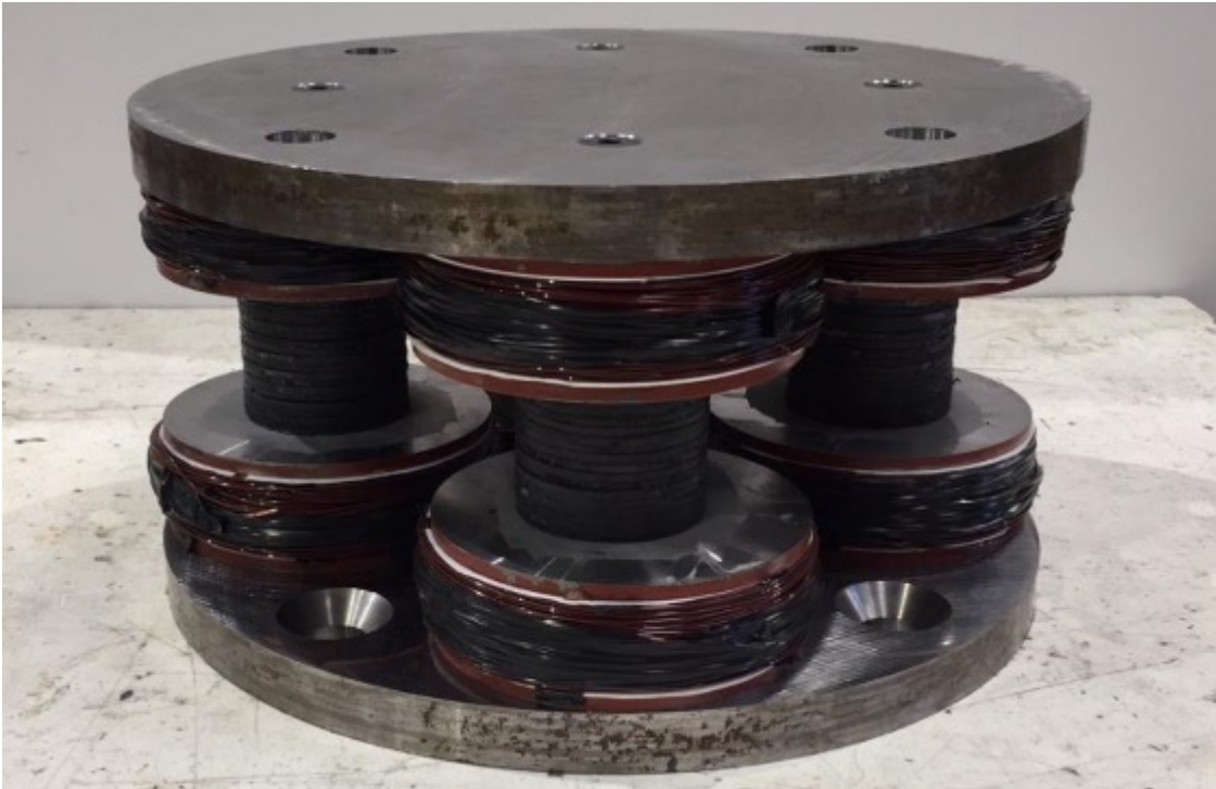
Figure 2. A prototype of the adaptive bridge bearing system. © University of Nevada, Reno
