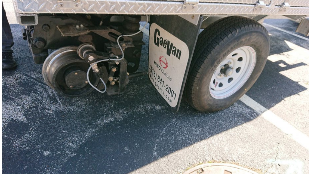
Figure 3 – Optical Encoder (attached to rail wheel)
