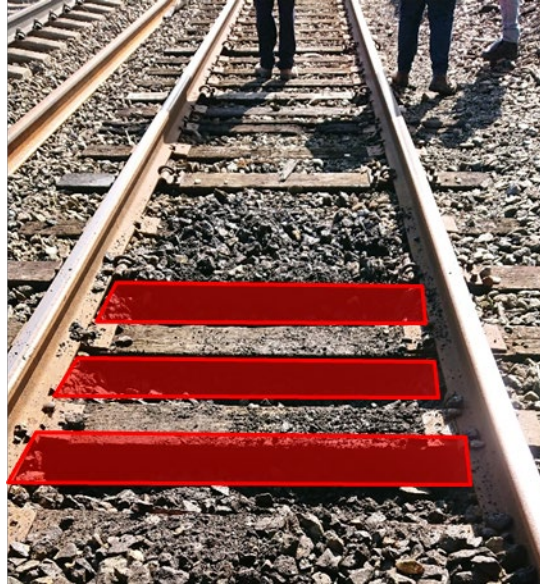
Figure 17 – Ballast-in-Crib Height Measurements
