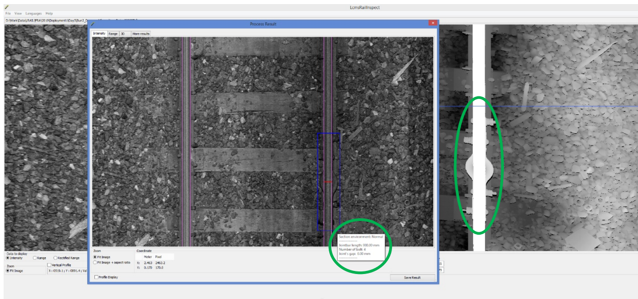
Figure 55 – Right Rail at MP 22+3076 with Four Bolts (D2R1)
