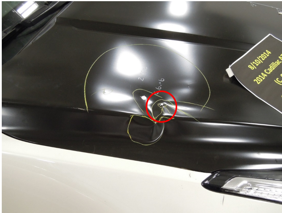
Figure 15. Strut tower bolt intrusion (circled in red) in the Cadillac ATS at impact location (C,6,+6)
