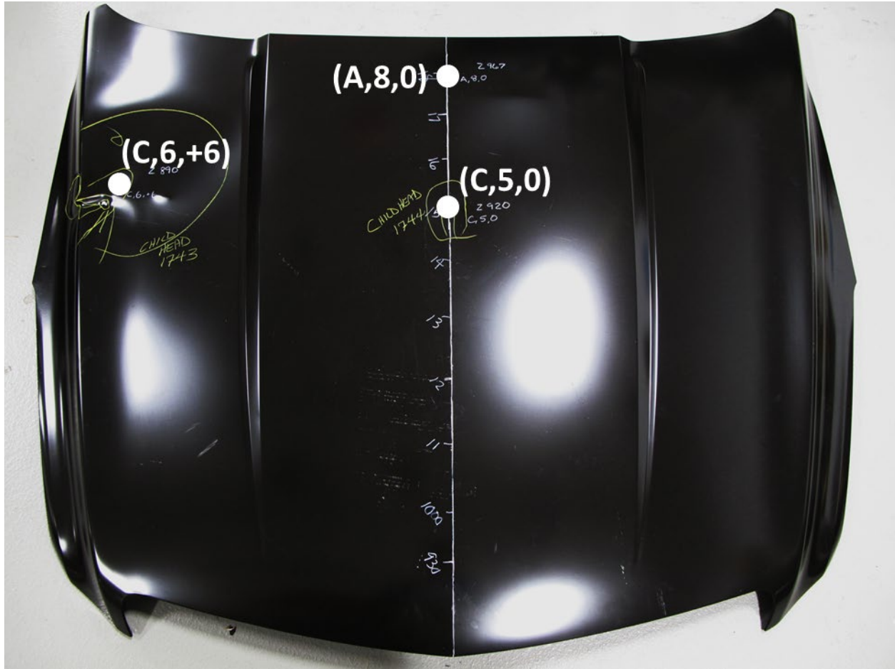
Figure 12. 2014 Cadillac ATS headform impact points
