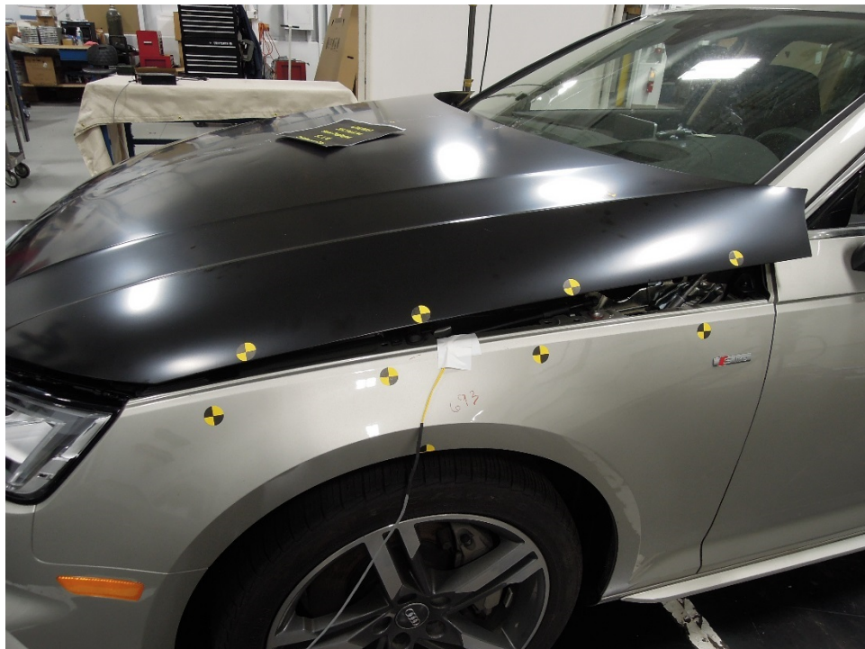
Figure 11. 2017 Audi A4 deployed-static hood. Upon deployment, the hood slides rearward and extends upward.
