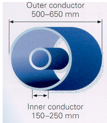
Figure 54: Cross Section of Siemens GIL
